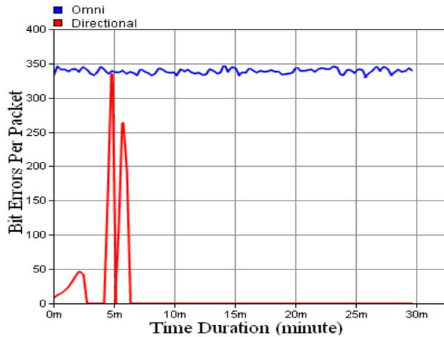
Figure 3. Radio Receiver Bit Error Per Packet Vs Time Duration
