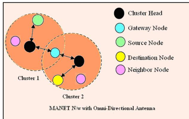
Figure 1. Showing the Previous approach having Cluster Head, Cluster Gateway and Cluster Nodes with Omni-Directional antenna.
