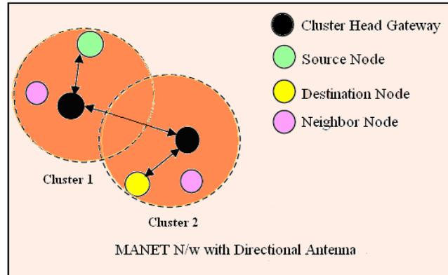
Figure 2. Showing the Current approach having Cluster Head Gateway (CHG) and Cluster Nodes with Directional antenna.
