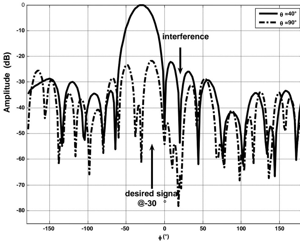
Figure 8. Planar antenna array pattern with main beam at  $(\varphi=-30, \theta=40^\circ)$  and one null at  $(\varphi=20^\circ, \theta=90^\circ)$
