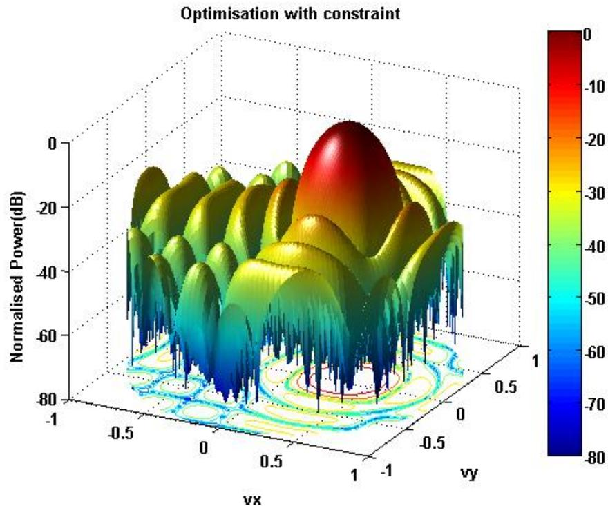
Figure 5. Planar antenna array pattern with main beam at  $(\varphi=5^\circ, \theta=20^\circ)$  and one null at  $(\varphi=-155^\circ, \theta=80^\circ)$
