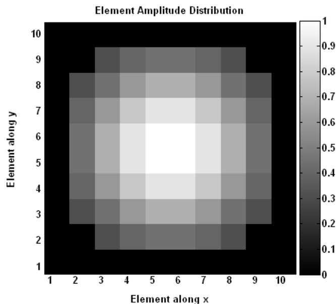
Fig. 4. The element excitation required to achieve the desired pattern ( $10 \times 10$  equispaced isotropic elements) given with the Chebyshev method.
