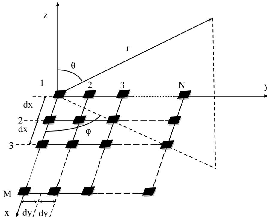
Figure 1. The structure of an  $M \times N$  element radiation antenna array.
