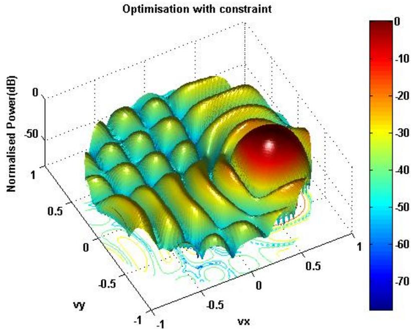
Figure 7. Planar antenna array pattern with main beam at  $(\varphi=-30, \theta=40^\circ)$  and one null at  $(\varphi=20^\circ, \theta=90^\circ)$
