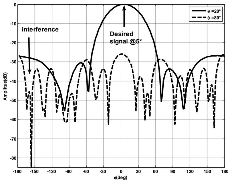
Figure 6. Planar antenna array pattern with main beam at  $(\varphi=5^\circ, \theta=20^\circ)$  and one null at  $(\varphi=-155^\circ, \theta=80^\circ)$
