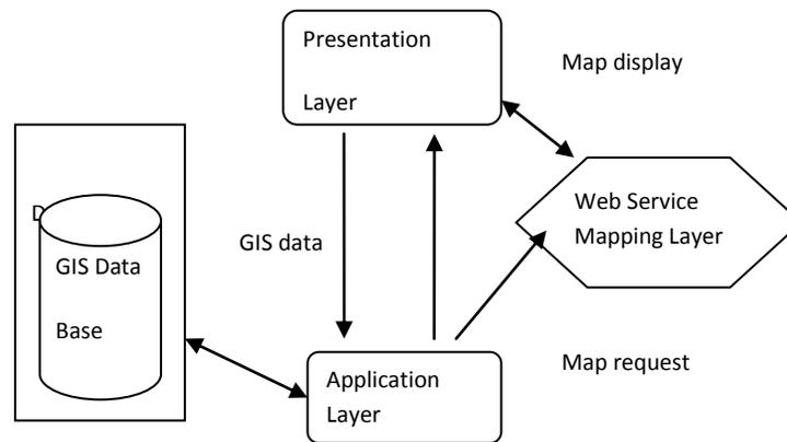
Figure 2 Web-based GIS Architecture (Peng and Tsou, 2003)
