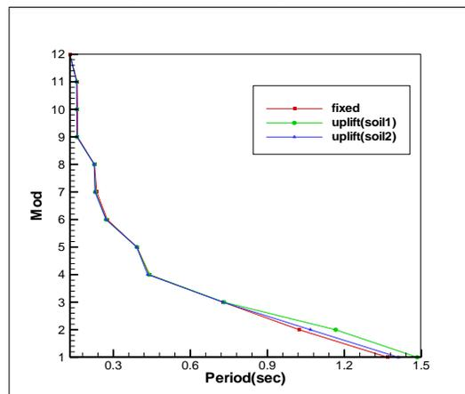
Figure 7 – Period for twelve-story structure with EBF system
