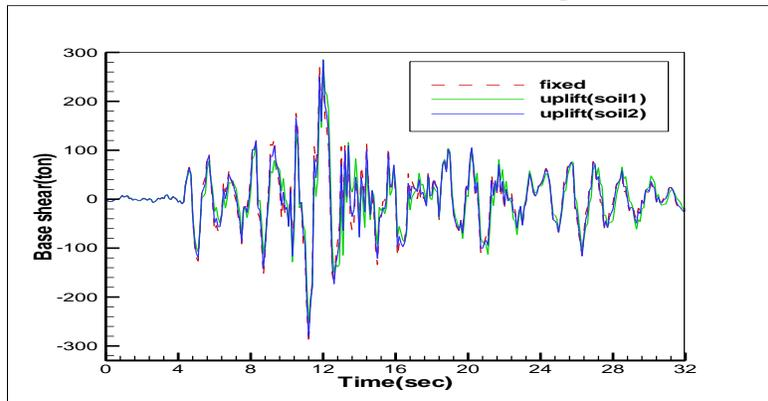
Figure 8 – Base shear for twelve-story structure with CBF system
