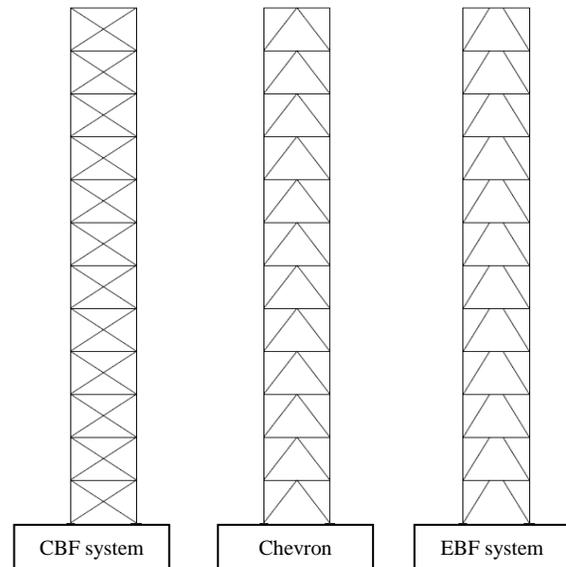
Figure 2 - Structural Systems in height
