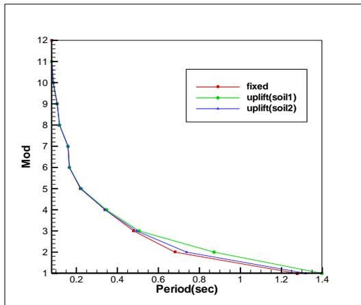
Figure 5 – Period for twelve-story structure with CBF system
