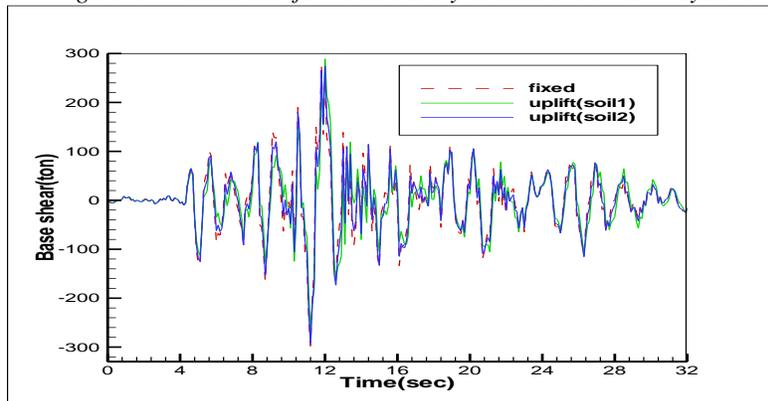
Figure 9 – Base shear for twelve-story structure with chevron system
