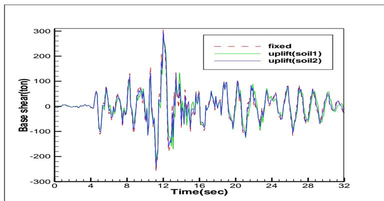
Figure 10 – Base shear for twelve-story structure with EBF system
