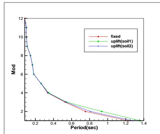
Figure 6 – Period for twelve-story structure with chevron system
