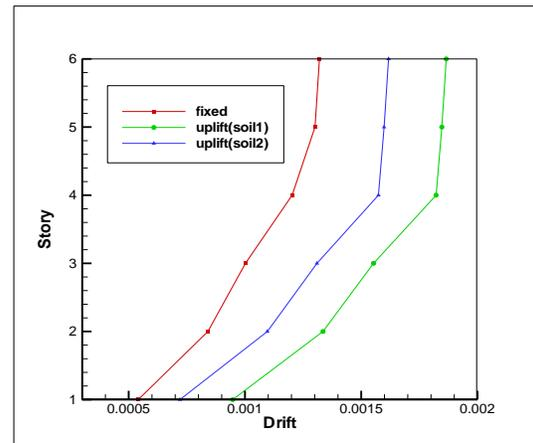
Figure 11 – Story drift ratio for three-story structure with CBF system    Figure 12 – Story drift ratio for six-story structure with chevron system
