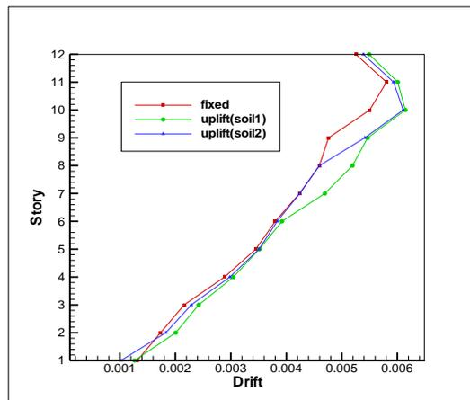
Figure 13 – Story drift ratio for twelve-story structure with EBF system
