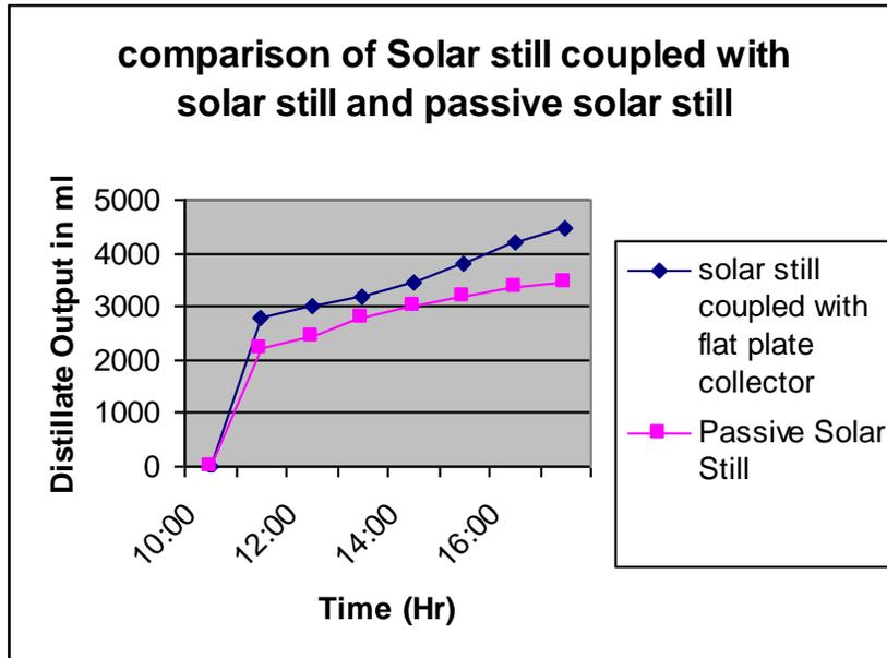
Fig.4. comparison of alone solar still versus solar still coupled with flat plate collector
