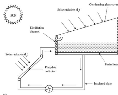
Fig.2. Schematic Arrangement of Solar still coupled with flat plate collector
