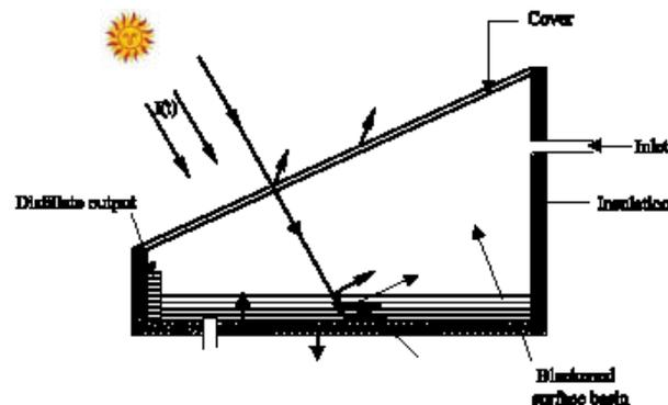
Fig.1. Schematic Diagram of Solar Still
