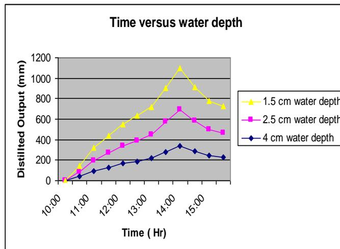
Fig.5. Effect of water depth on solar still productivity
