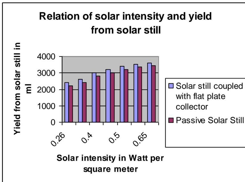
Fig.3. Relation of solar intensity and solar still distillate output during August, 2010
