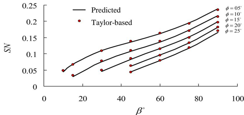
Figure 3 Comparison of Taylor-based stability numbers with those predicted using the proposed regression formula
