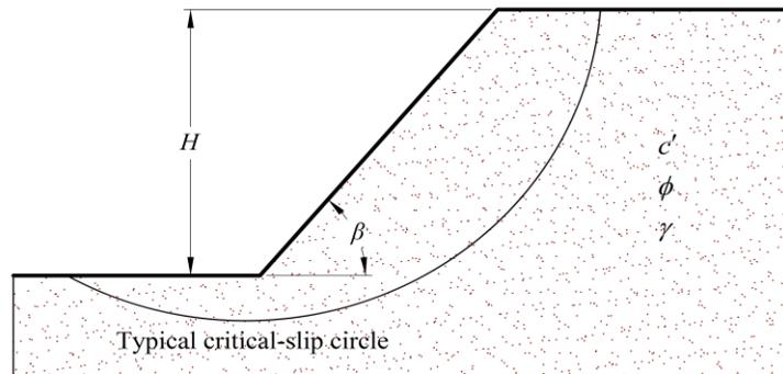
Figure 2 slope geometry along with a typical critical-slip circle
