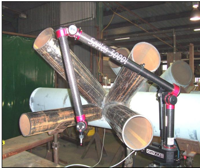
Figure 2. Fabrication of cluster A11 specimen S2.
