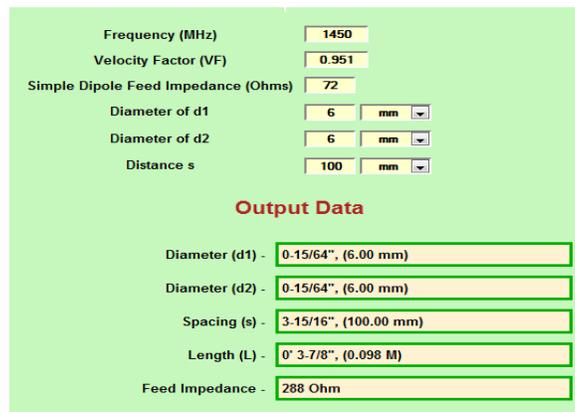
**Figure 2: Showing the input and output data in the K7MEM Folded Dipole Antenna Online Simulator (<http://www.dxzone.com/cgi-bin/dir/jump2.cgi>)**
