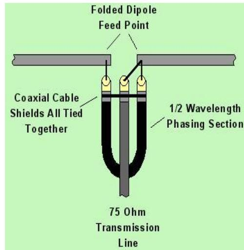
Figure 5: Showing the antenna matching technique with the 75Ω coaxial cable.
