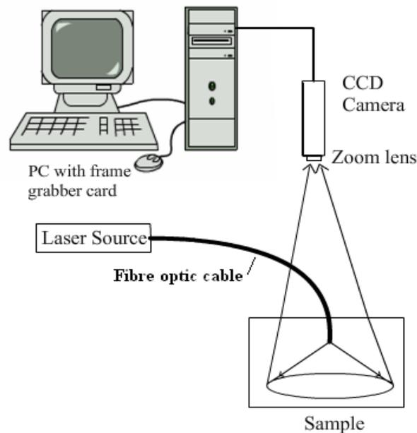
Figure 7. Experimental setup for laser speckle imaging
