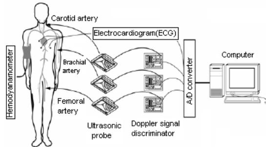
Figure 3. Ultrasound velocimeter system for simultaneous measurement in multiple arteries (Reproduced by permission of IEEE, Piscataway, NJ (© 2004 IEEE), from Azran et al. <sup>25</sup>)
