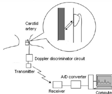
Figure 2. Ultrasound based blood flow measurement system (Reproduced by permission of IEEE, Piscataway, NJ (© 2005 IEEE), from Yamaguchi et al.<sup>24</sup>)
