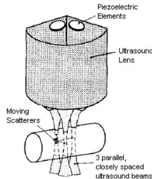
Figure 6. 3-D flow velocity vector measurement concept using Ultrasound (Reproduced by permission of IEEE, Piscataway, NJ (© 1995 IEEE), from Ilmar et al. <sup>34</sup>)
