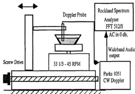
Figure 4. Experimental schematic for CW Doppler ultrasound system for microcirculation measurement (Reproduced by permission of IEEE, Piscataway, NJ (© 1997 IEEE), from David et al. <sup>27</sup>)
