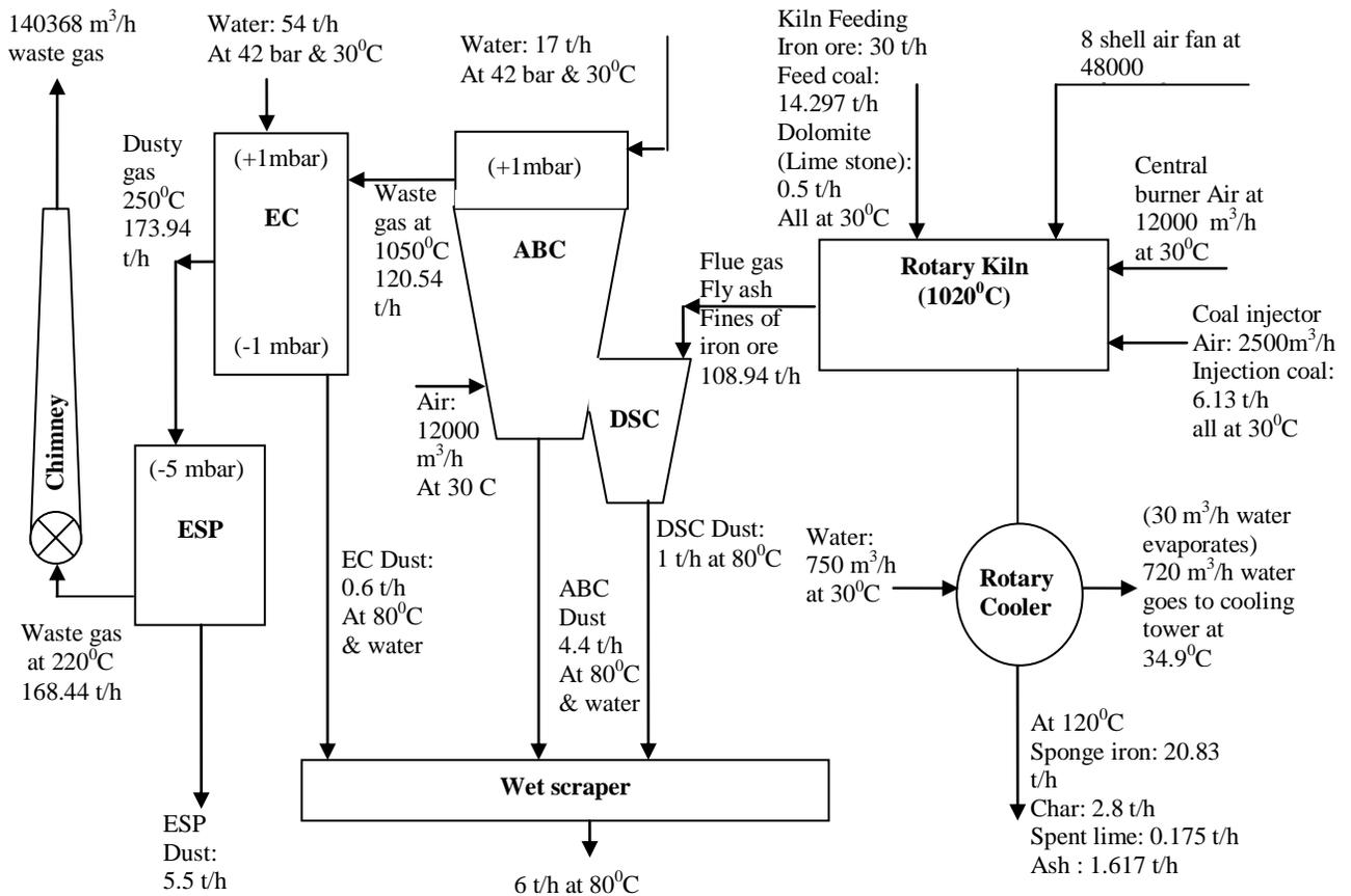
Figure 1. Conventional sponge iron plant flow diagram
