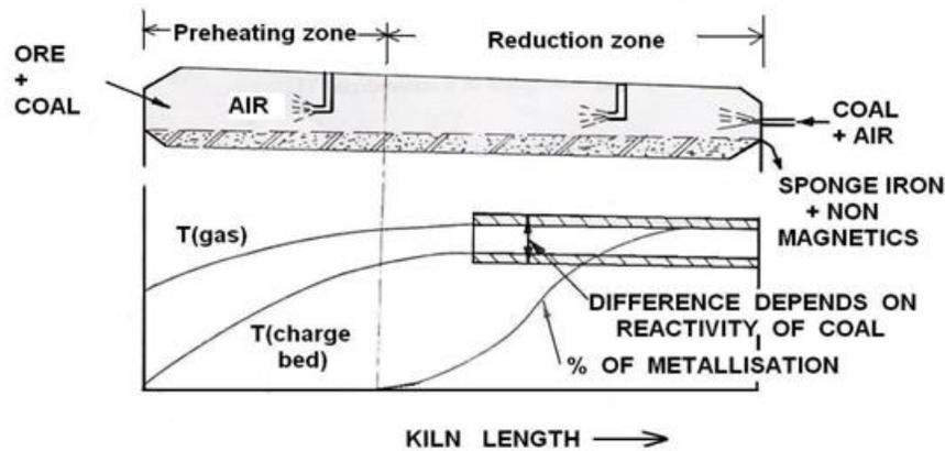
Figure 2. Principle of counter kiln operation
