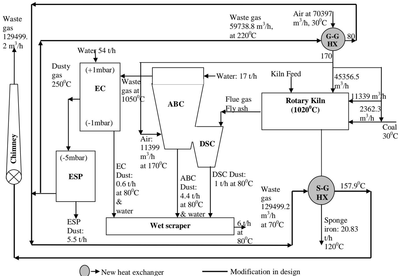
Figure 4. Process flow diagram for Case-3
