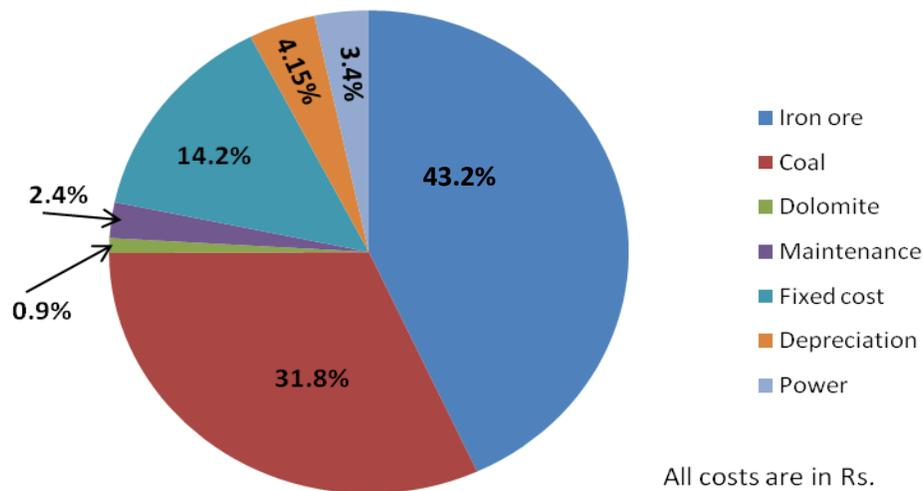
Figure 3. Cost components for one tonne production of Sponge iron
