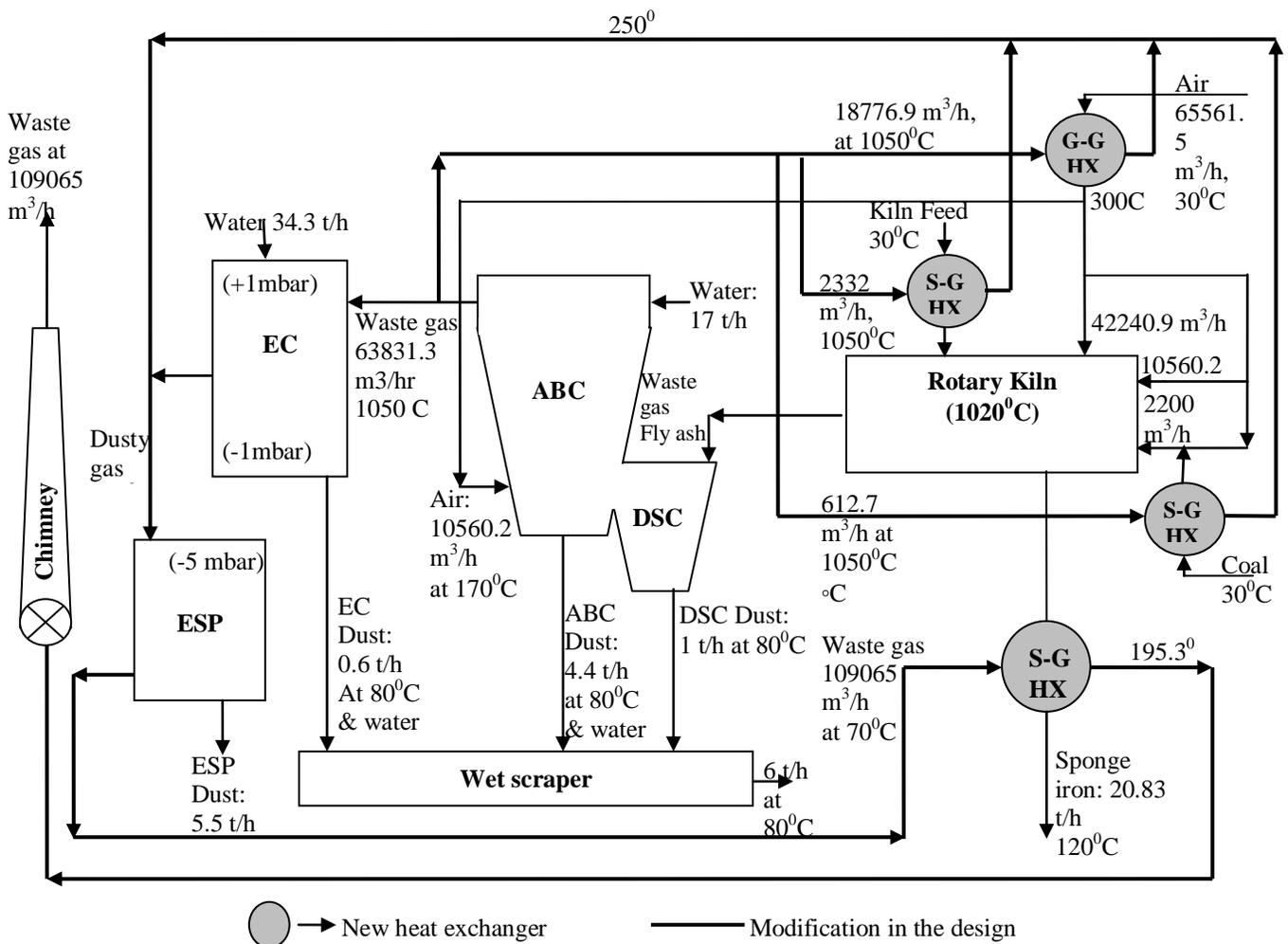
Figure 6. Process flow diagram for Case-4
