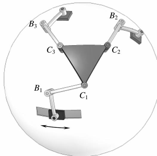
Fig. 7. A direct kinematic singularity of a 4-ADOFs redundant spherical parallel manipulator with four revolute active joints.
