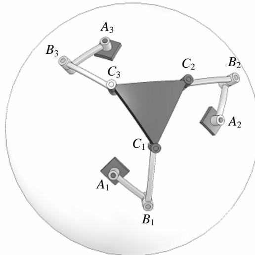
Fig. 1. 3-RRR spherical parallel manipulator.
