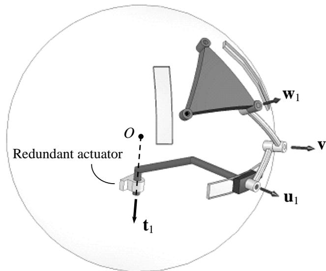
Fig. 4. One leg of the manipulator.
