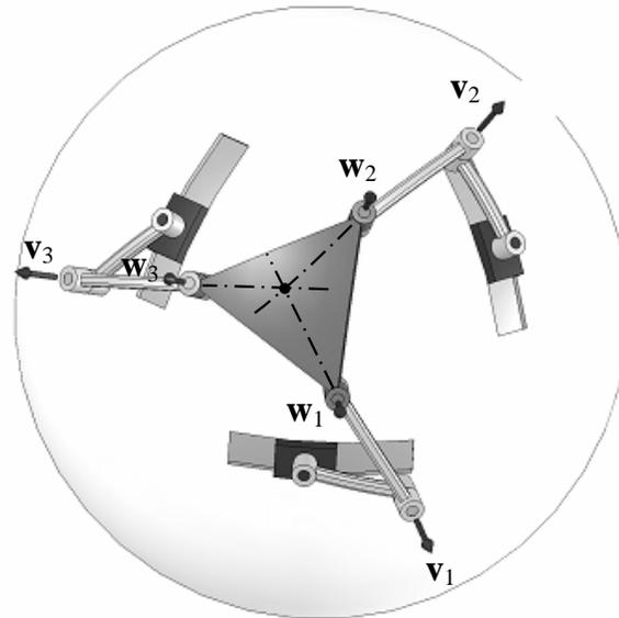
Fig. 6. A direct kinematic singularity of spherical 3-RRR manipulator in which planes of the distal links intersect at a common line.
