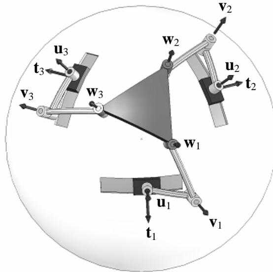
Fig. 3. The 3-RRR kinematically redundant spherical parallel manipulator.
