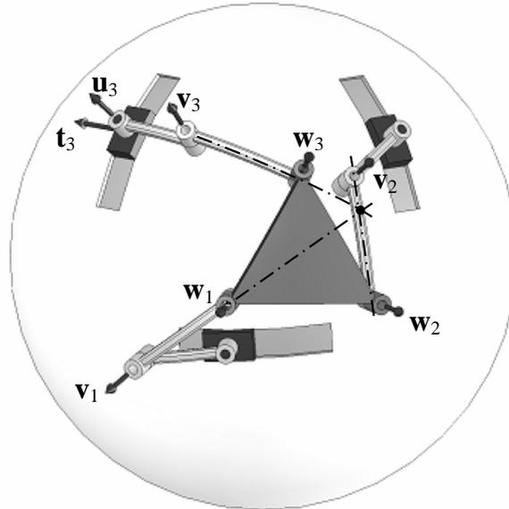
Fig. 8. A combined singularity of the spherical 3-RRR manipulator where the two first singularities occur simultaneously.
