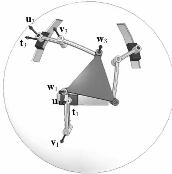
Fig. 5. An inverse kinematic singularity of spherical 3-RRR manipulator in which legs one and three are in branch-singular poses.
