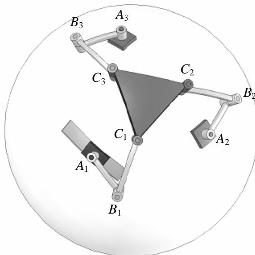
Fig. 2. A 4-ADOFs kinematically redundant spherical parallel manipulator (2-RRR+1-PRRR).
