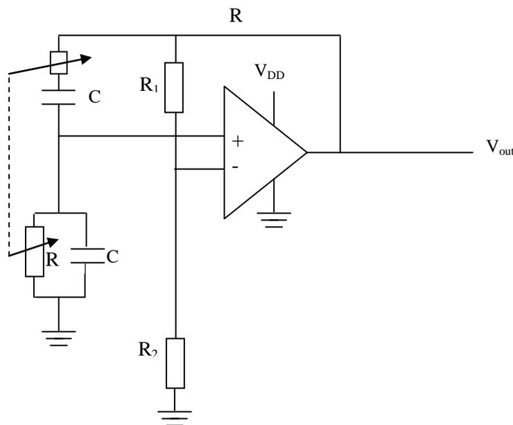
**Figure 4:** Wien-bridge oscillator circuit.
