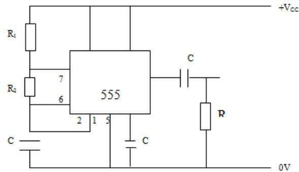
**Figure 9:** Integrated Circuit (using 555 timer) Astable Multivibrator oscillator.
