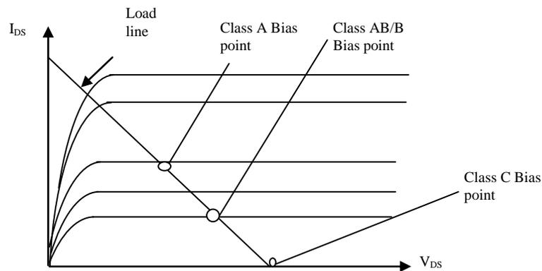
**Figure 13:** Showing the operation of transconductance amplifier classes
