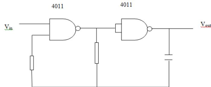
**Figure 11:** Gated CMOS oscillator circuit.
