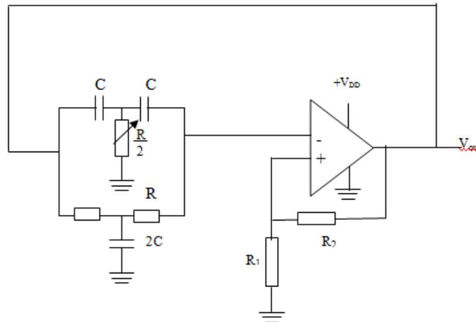
**Figure 5:** Twin-T oscillator circuit.
