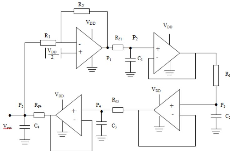
**Figure 6:** Bubba oscillator circuit.
