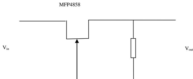
**Figure 10:** JFET Chopper oscillator circuit.
