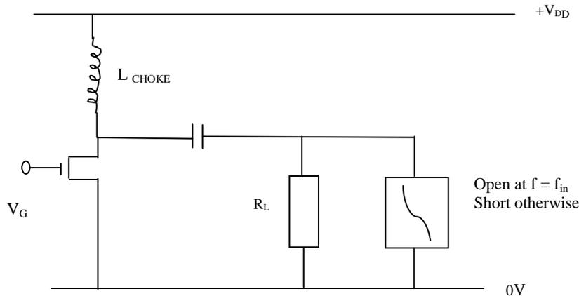
Figure 12: Showing simple circuit diagram of a transconductance amplifier.
