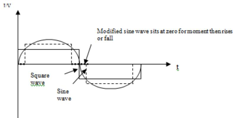
**Figure 2:** Showing a.c output of the sine wave, square wave and modified sine wave inverters.
