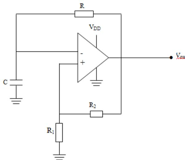
Figure 7: Relaxation oscillator circuit.
