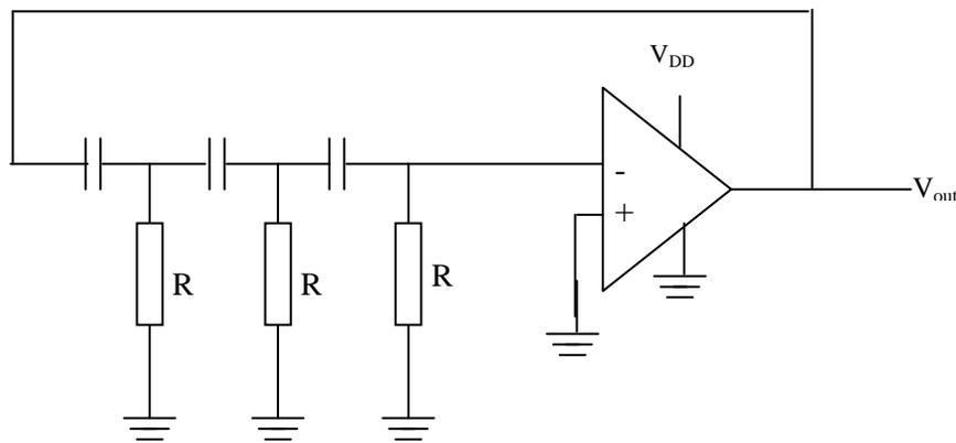
**Figure 3:** Phase –shift oscillator with three lead circuits.
