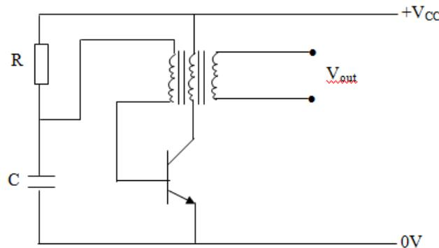
Figure 8: Blocking oscillator circuit.
