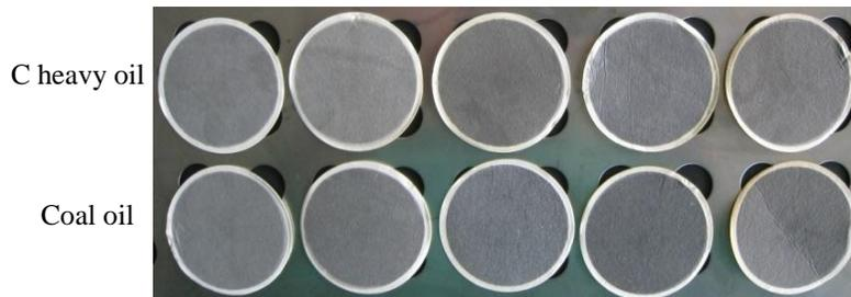
Figure 5. Filter for particulate measurement
