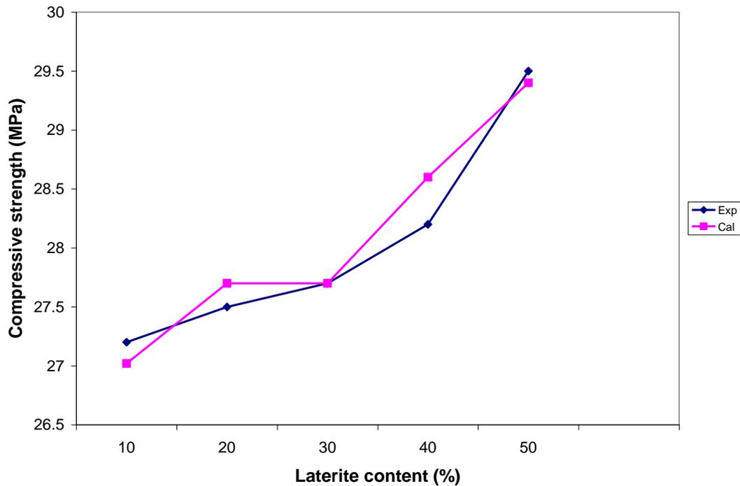
Fig.5 Comparison of experimental and calculated 28-day compressive strength of laterized concrete
