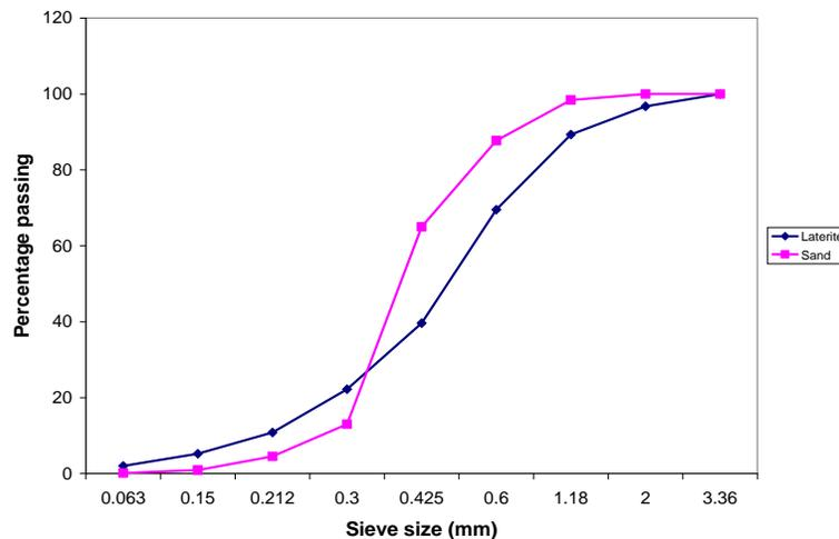
Fig.1. Grain-size distribution of laterite and sand
