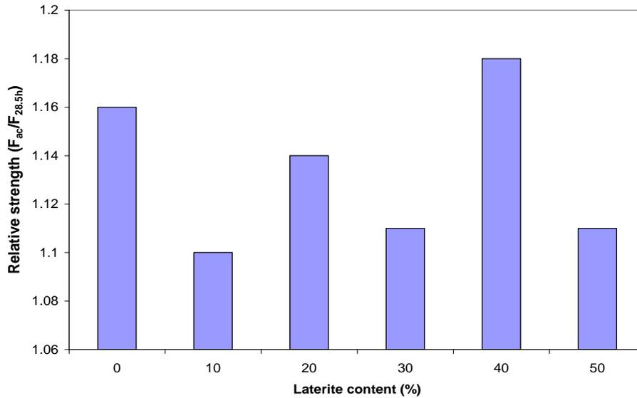
Fig. 2. Accelerated strength relative to 28.5 h strength of laterized concrete
