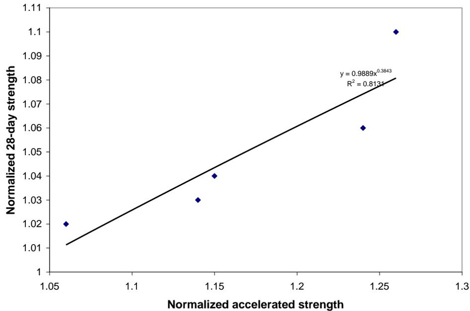
Fig. 4. Normalized accelerated strength versus normalized 28-day strength of laterized concrete
