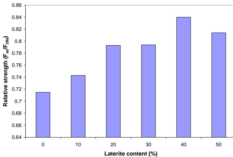
Fig. 3. Accelerated strength relative to 28-day strength of laterized concrete
