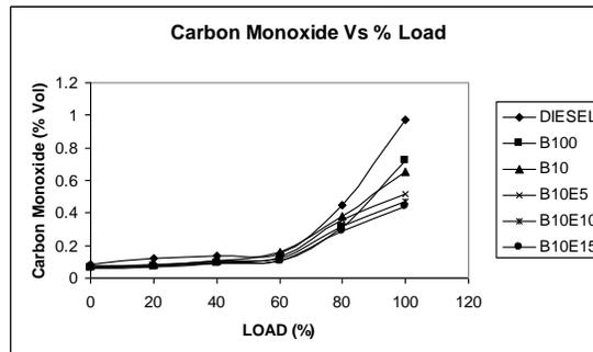
Figure 6. Variation of carbon monoxide emissions with Load
