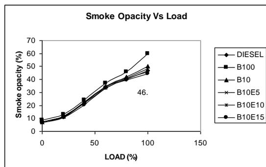
Figure 11. Variation of smoke opacity with Load
