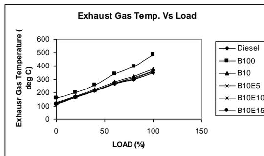
Figure 4. Variation of exhaust gas temperature with Load
