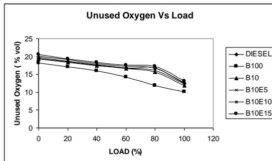
Figure 10. Variation of unused oxygen with Load.
