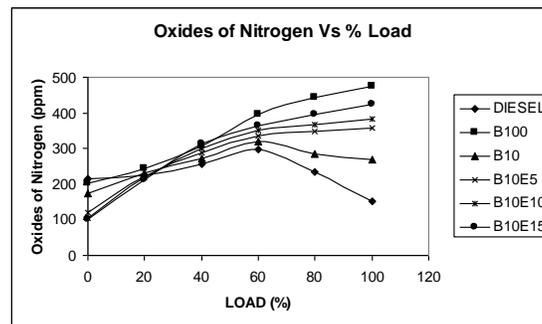
Figure 8. Variation of oxides of nitrogen with Load.
