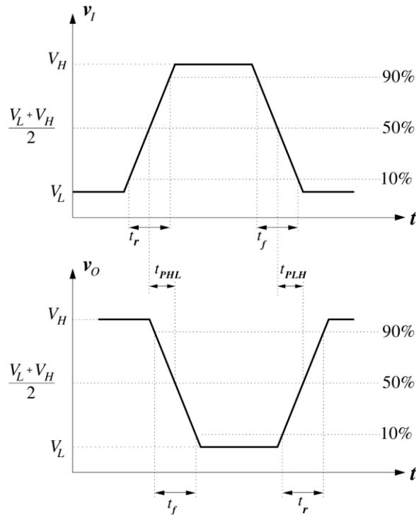
Figure 10. Time and voltage definitions for input and output waveforms [19].
