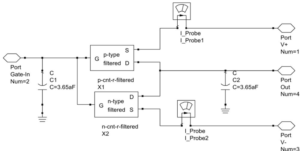
Figure 4. Schematic of a NOT gate.
