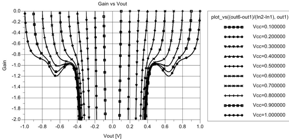
Figure 9. Gain of the first NOT of the cascade vs  $V_{out}$  with  $V_{CC}$  varying from 0.1 V to 1.0 V, step 0.1.
