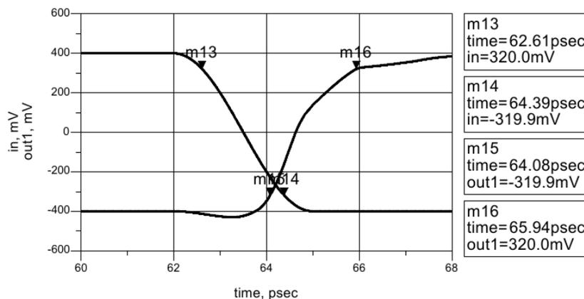
Figure 15. Input and output of transients of the first NOT gate for low-to-high transitions.
