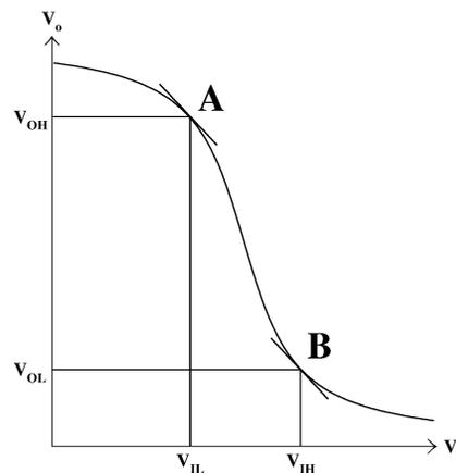
Figure 3. Voltage transfer characteristic for an inverter.
