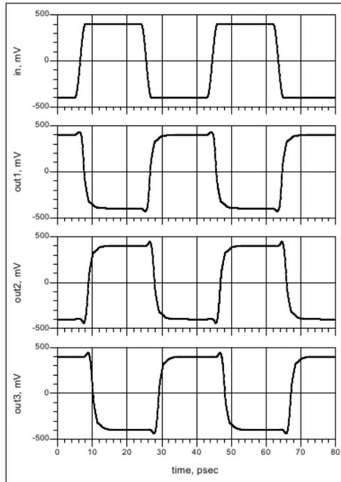
Figure 11. Output of the first four NOT gates and input signal vs time for slow transitions.
