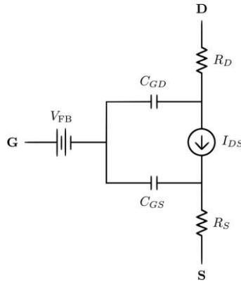
Figure 1. Equivalent Circuit of a n-type CNTFET [2-3].
