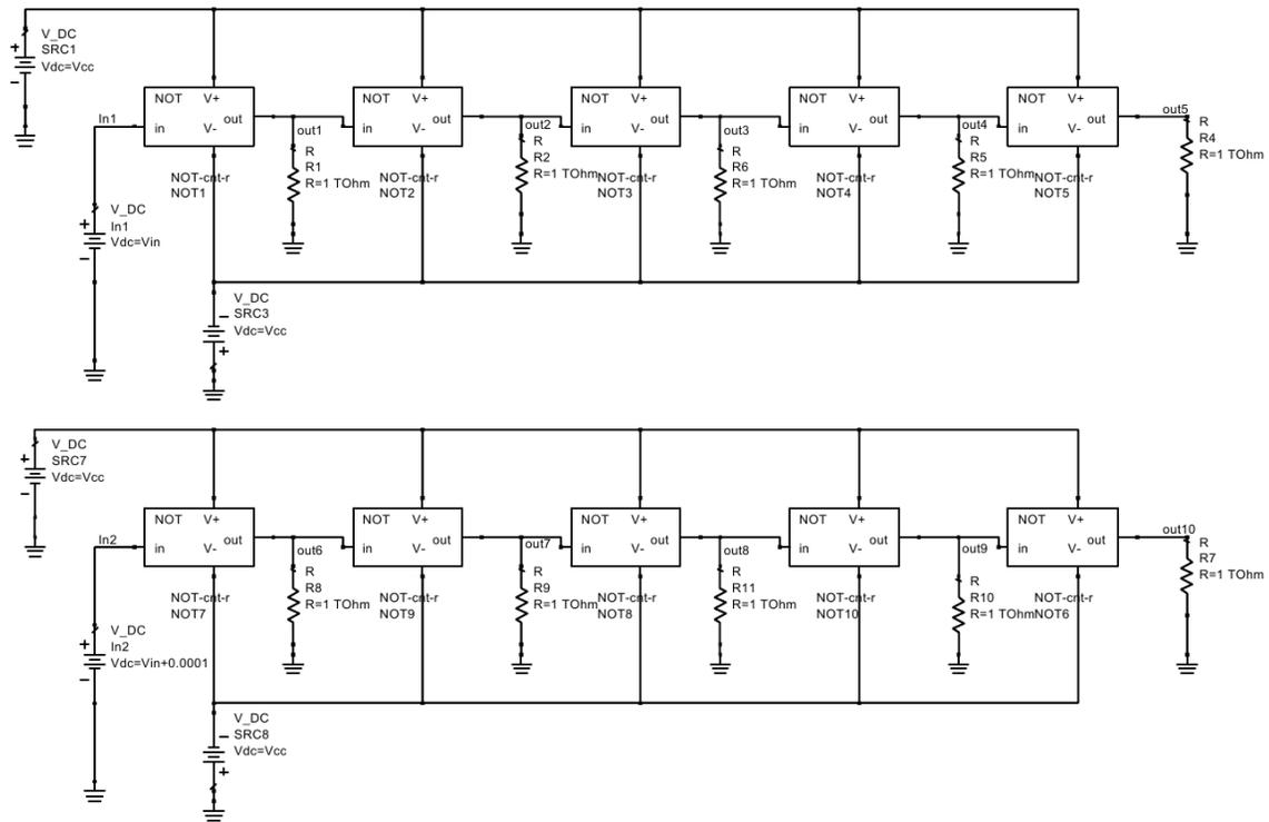
Figure 7. Circuit used to calculate NOT gain.
