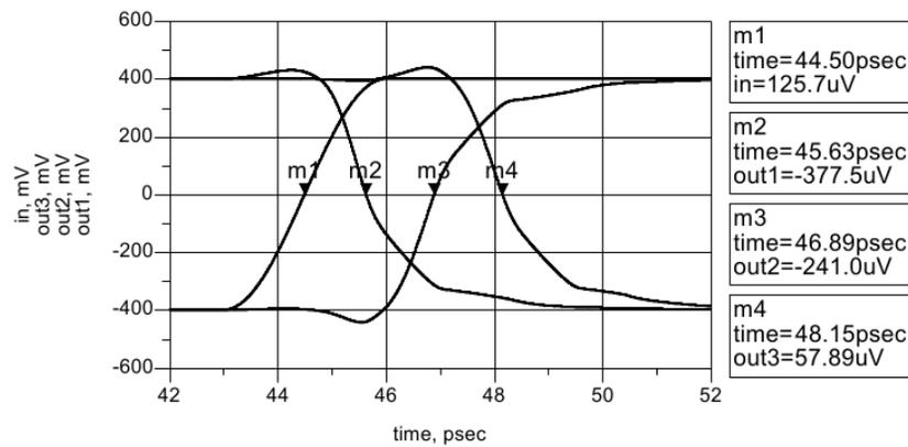
Figure 12. Input and output of transients of the NOT gates for high-to-low transitions.
