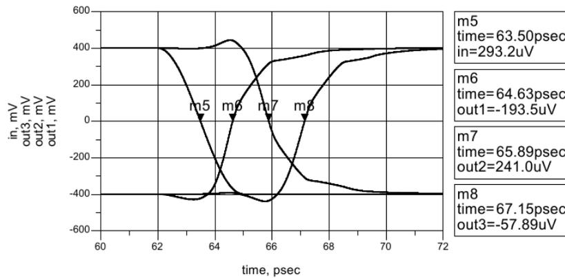
Figure 13. Input and output of transients of the NOT gates for low-to-high transitions.
