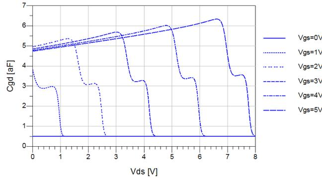
Figure 2a. Simulations of  $C_{GD}$  vs  $V_{DS}$  for different values of  $V_{GS}$  in Verilog-A.
