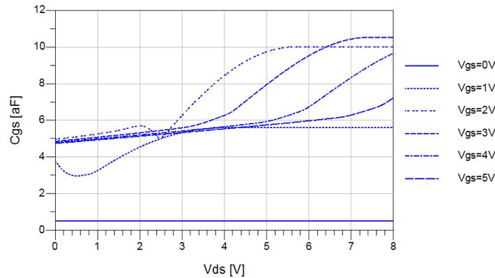
Figure 2b. Simulations of  $C_{GS}$  vs  $V_{DS}$  for different values of  $V_{GS}$  in Verilog-A.
