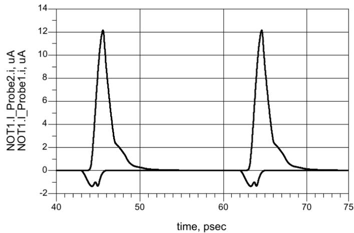
Figure 16. Dynamic currents flowing through the first NOT gate (our model).
