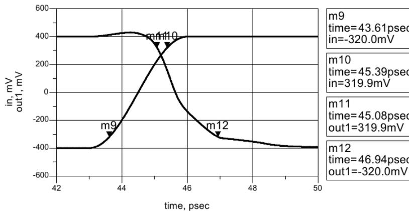
Figure 14. Input and output of transients of the first NOT gate for high-to-low transitions.
