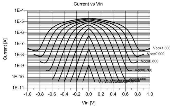
Figure 6. Static currents of the first NOT gate vs  $V_{in}$ , with  $V_{cc}$  varying from 0.1 V to 1.0 V.
