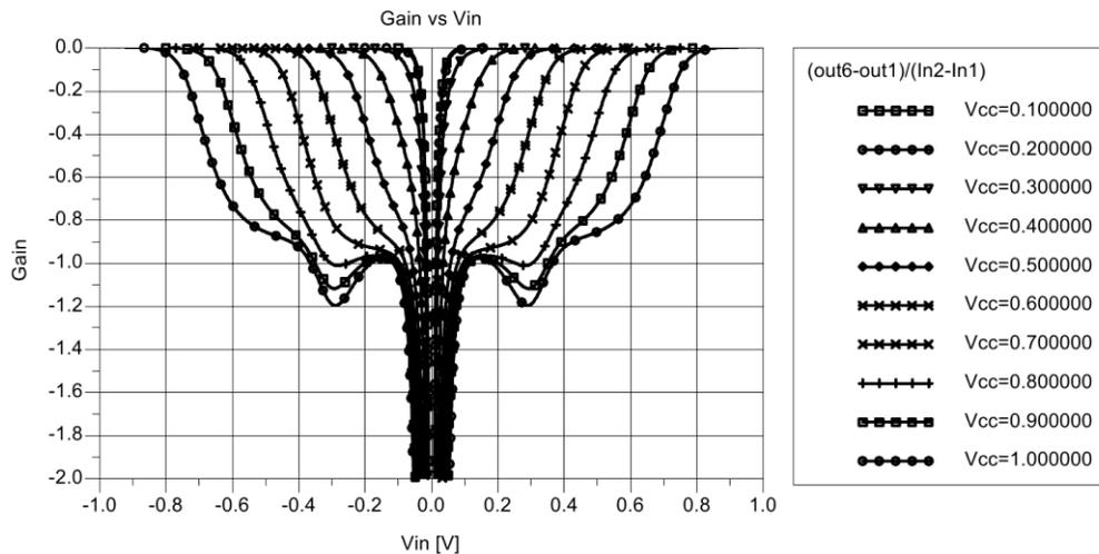
Figure 8. Gain of the first NOT of the cascade vs  $V_{in}$  with  $V_{CC}$  varying from 0.1 V to 1.0 V.
