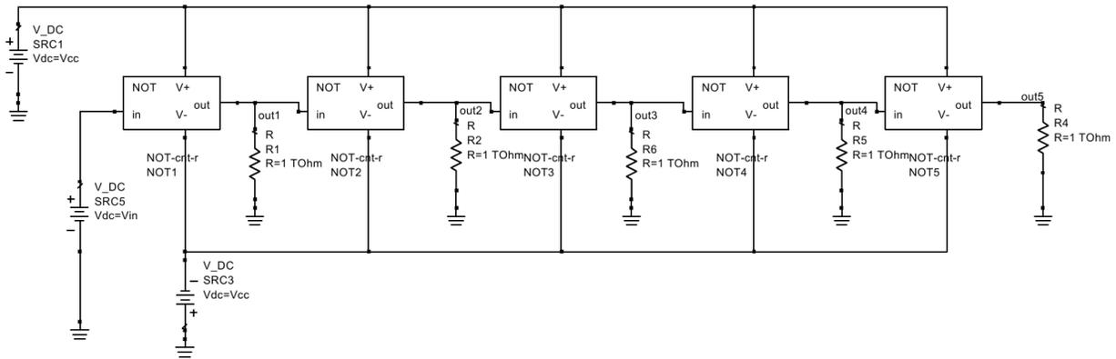
Figure 5. Schematic of a cascade of five NOT gates.
