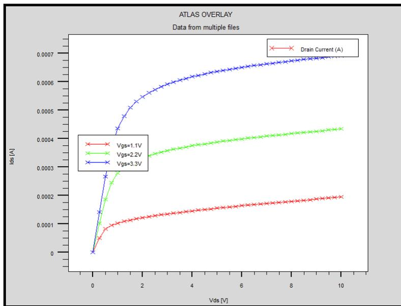
Figure 5.  $I_{ds}$ - $V_{ds}$  characteristics using a boron dose  $8 \cdot 10^9 \text{ cm}^{-2}$ .
