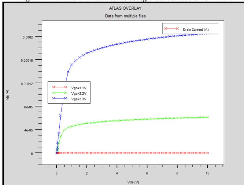
Figure 2.  $I_{ds}$ - $V_{ds}$  characteristics using a boron dose  $8 \cdot 10^{13} \text{ cm}^{-2}$ .
