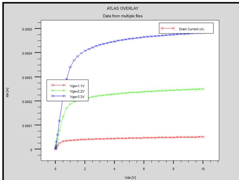
Figure 1.  $I_{ds}$ - $V_{ds}$  characteristics using a boron dose  $8 \cdot 10^{12} \text{ cm}^{-2}$ .
