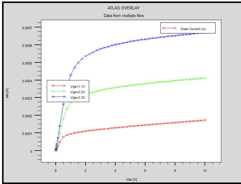
Figure 4.  $I_{ds}$ - $V_{ds}$  characteristics using a boron dose  $8 \cdot 10^{10} \text{ cm}^{-2}$ .
