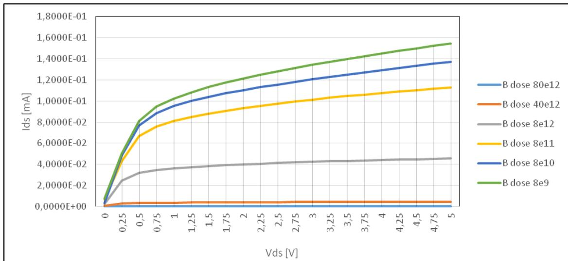
Figure 6.  $I_{ds}$ - $V_{ds}$  characteristics using the considered boron doses for  $V_{gs} = 1.1$  V.
