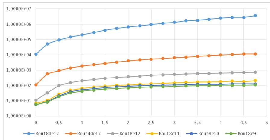
Figure 7.  $R_{out}$ - $V_{ds}$  characteristics using the considered boron doses for  $V_{gs} = 1.1$  V.
