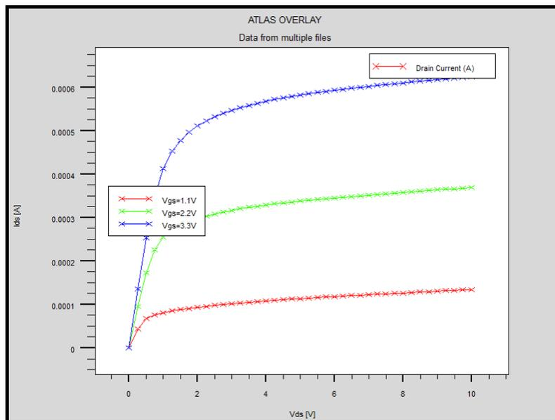
Figure 3.  $I_{ds}$ - $V_{ds}$  characteristics using a boron dose  $8 \cdot 10^{11} \text{ cm}^{-2}$ .
