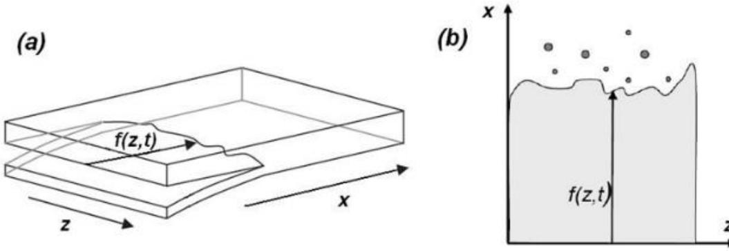
Figure 1. Geometry of the fracturing system: (a) Sketch of the experimental fracture test where an interfacial crack is made propagate at the weak interface between two elastic plates; (b) Schematic view of the heterogeneous interface where the crack front deforms under the effect of heterogeneities.
