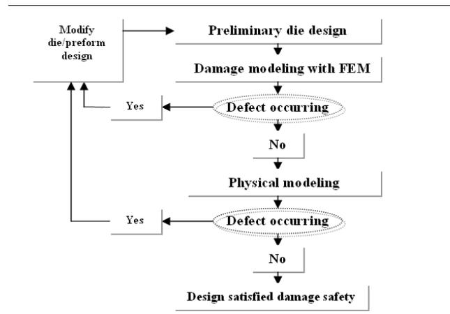
Figure 7. The steps offered to avoid possible damage on the forged parts.
