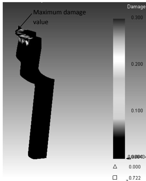
Figure 8. The regions that defects may occur according to damage modeling
