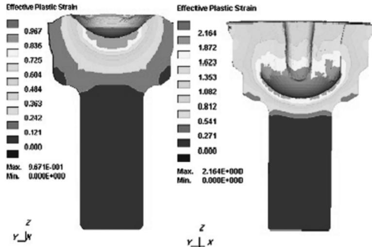
Figure 4. effective plastic strain in 50% of course and at the end of deformation
