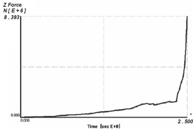
Figure 5. Load curve of close die forging
