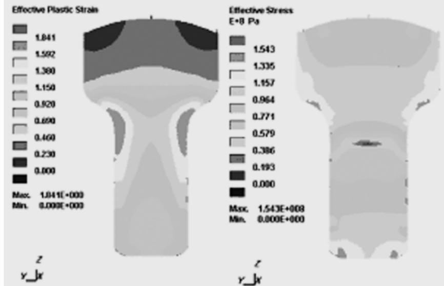
Figure 2. Effective plastic strain and stress at the end forward extrusion sequence
