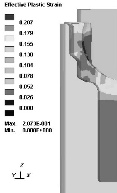
Figure 6. Configuration of tooling in ironing and effective plastic strain at the end of process
