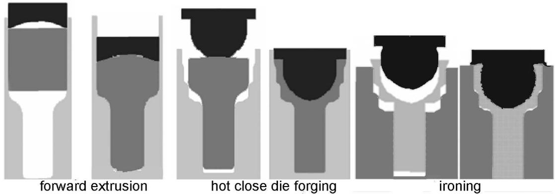
Figure 1. schematically shows the suggested multistage forging for a CV joint outer race
