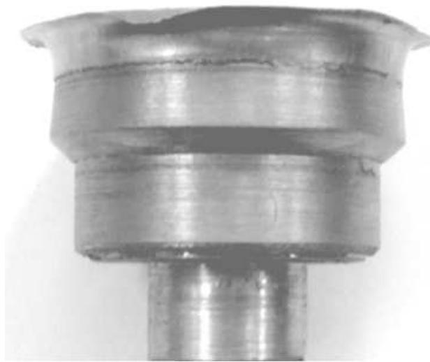
*Figure 10 shows a lead specimen with different pre-form geometry and none of mentioned surface defects are seen after ironing.*
