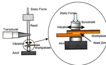
Figure 2. Ultrasonic welding [8]
