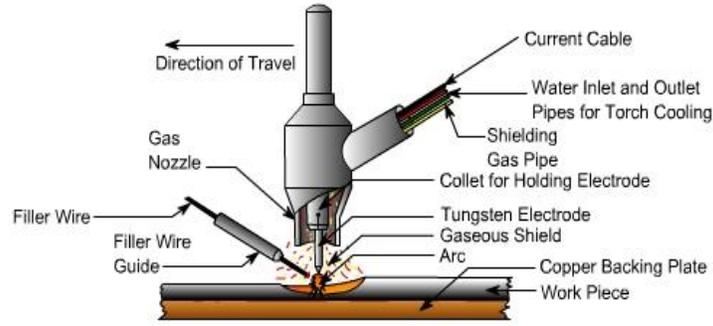
*Figure 4. Gas Tungsten Arc welding [7]*
