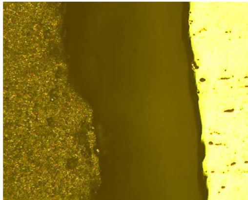
*Figure 6. Interface region of dissimilar metal weld joint [12]*
