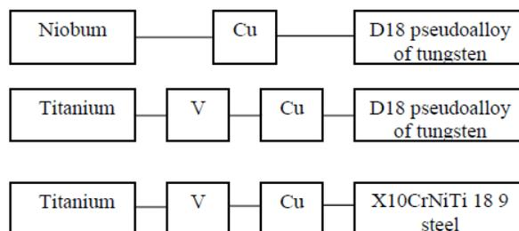
*Figure 7. Inter layering system in niobium and titanium joints [41]*
