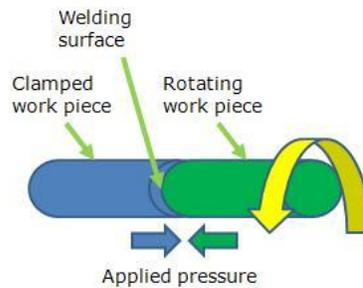
Figure 3. Friction welding [9]
