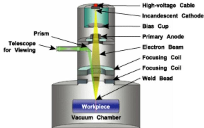
*Figure 5. Electron beam welding [7]*
