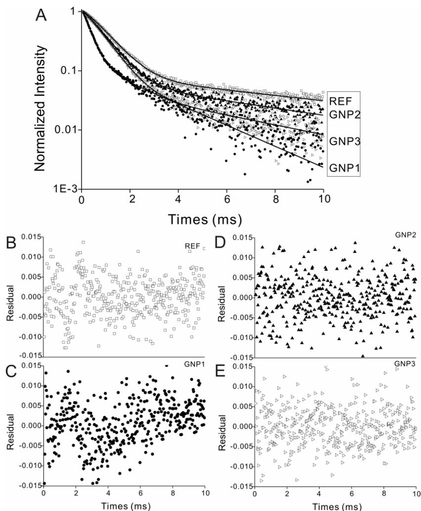
**Figure 4.** Observed Hahn echo decays of samples REF, GNP1, GNP2 and GNP3 acquired at 90C. REF represents a PPC reference sample and GNP1 - 3 are PPC composites containing 10wt% of different types of graphite Nano platelets. The solid curves represent non-linear least squares fits to Equation 9. The bottom figures (B – E) show the residual curves for each individual sample .
