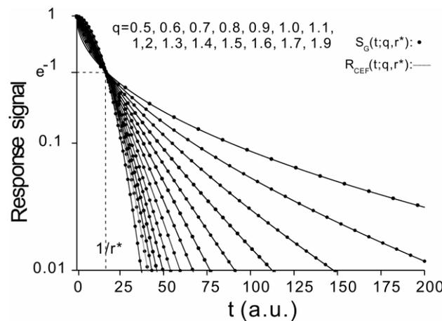
**Figure 2.** The integral function  $S_G(t; q, r^*)$  (equation 3) and the response function  $R_{CEF}(t; q, r^*)$  (equation 4a) as a function of time  $t$  for  $q$  (left to right) =  $0.50, 0.60, \dots, 1.60, 1.70$  and  $1.90$  and  $r$  set arbitrarily to  $0.065$ . All curves go through the point  $(1/r^*, e^{-1})$ .
