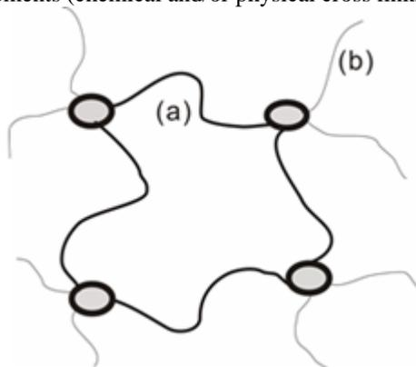
**Figure 3.** The graphite nano-platelets within a melt modified (PPC) composite introduce additional “cross-links” and/or entanglements (chemical and/or physical cross links).
