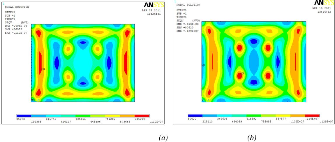
Fig.12. The stress contours of the mortar layer's surface in different working conditions
