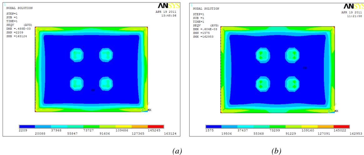
Fig.13. The stress contours on the internal side next to basal layer of the thermal insulation board
