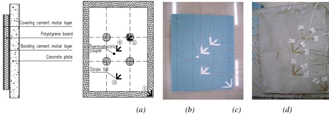
Fig. 3 Schematic diagram of the specimen
