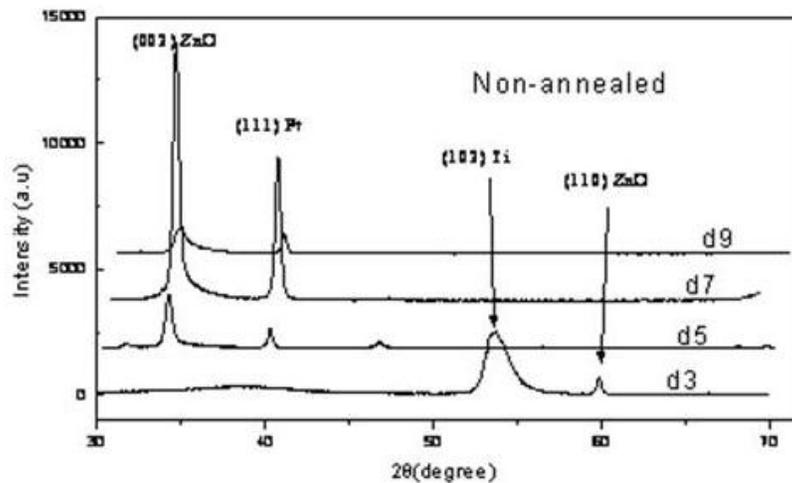
Figure 1a. XRD diagram from non annealed ZnO samples deposited on silicon substrates at different target to substrate distance.
