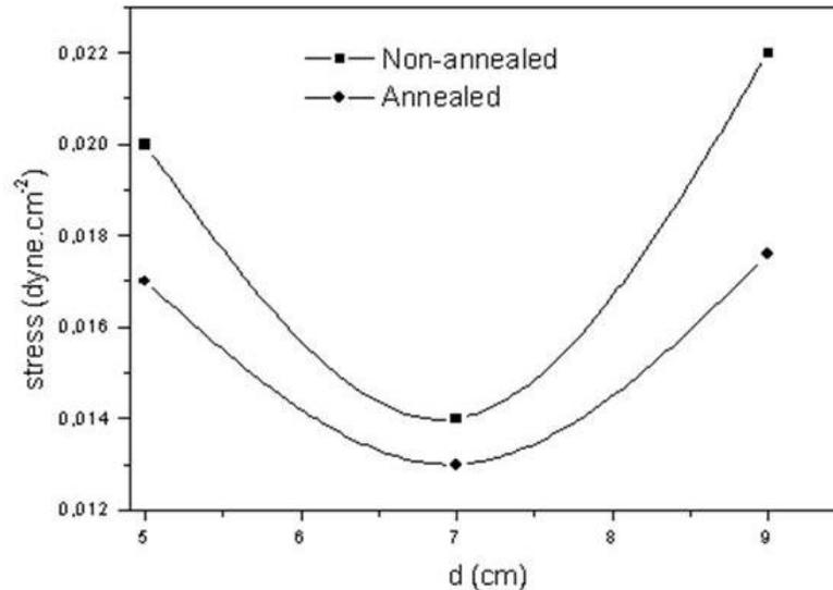
Figure 3. The variation of stress with respect to target to substrate distance of non annealed and annealed ZnO films.
