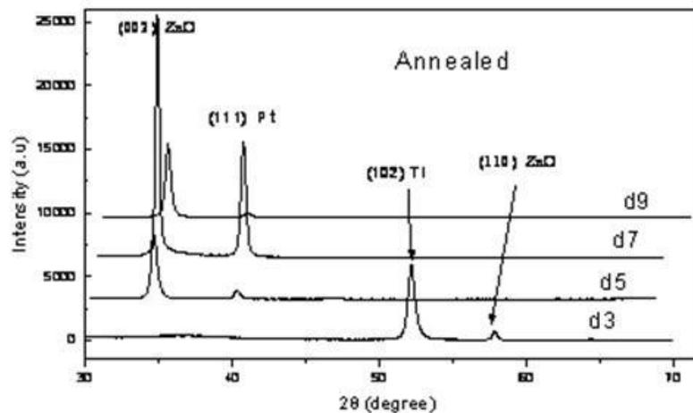
Figure 1b. XRD diagram from annealed ZnO samples deposited on silicon substrates at different target to substrate distance.
