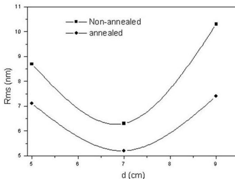
Figure 4. rms of ZnO films annealed and non annealed at different target to substrate distance.
