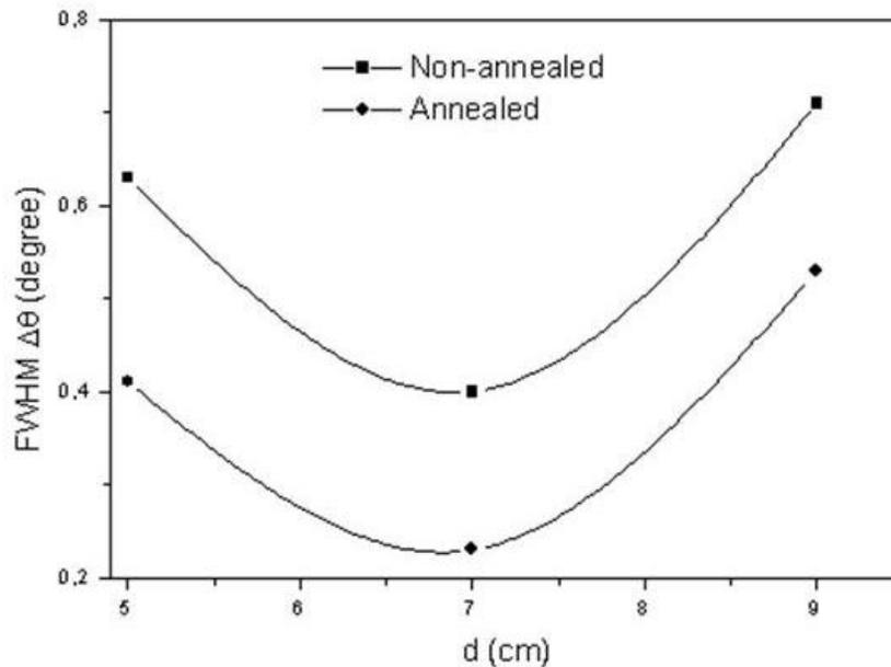
Figure 2. FWHM of (002) X-ray rocking curves for non annealed and annealed ZnO samples deposited on silicon substrates at different target to substrate distance.
