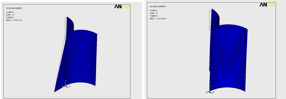
Figure 5. Structure elements for the finite element method (with and without counterfort shell retaining walls).
