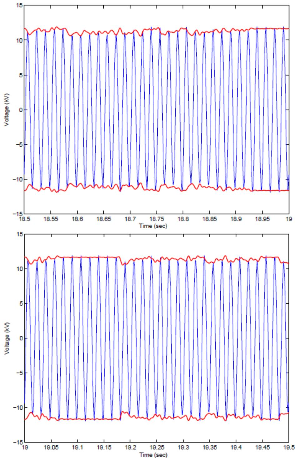
Figure 6. Estimated voltage envelope of an arc furnace signal
