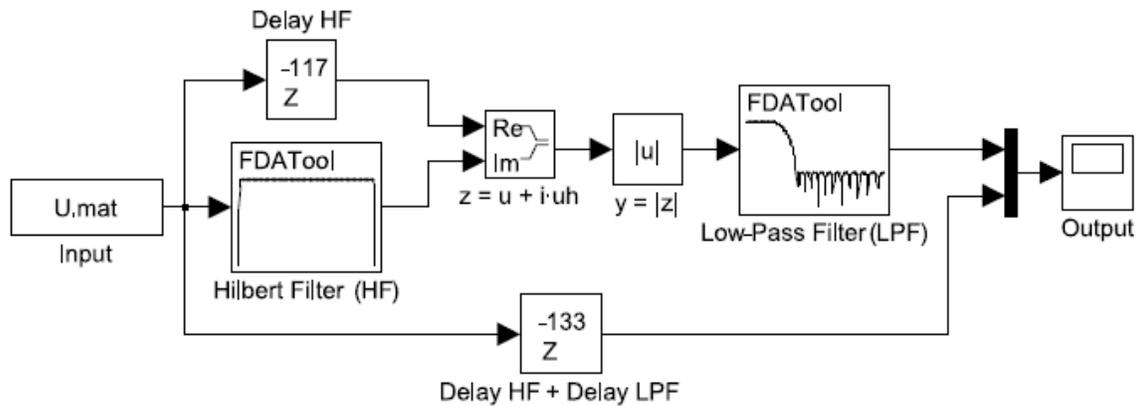
Figure 4. Block diagram for the estimator.
