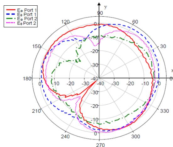
Figure 1. Radiation pattern of the PIFA element.
