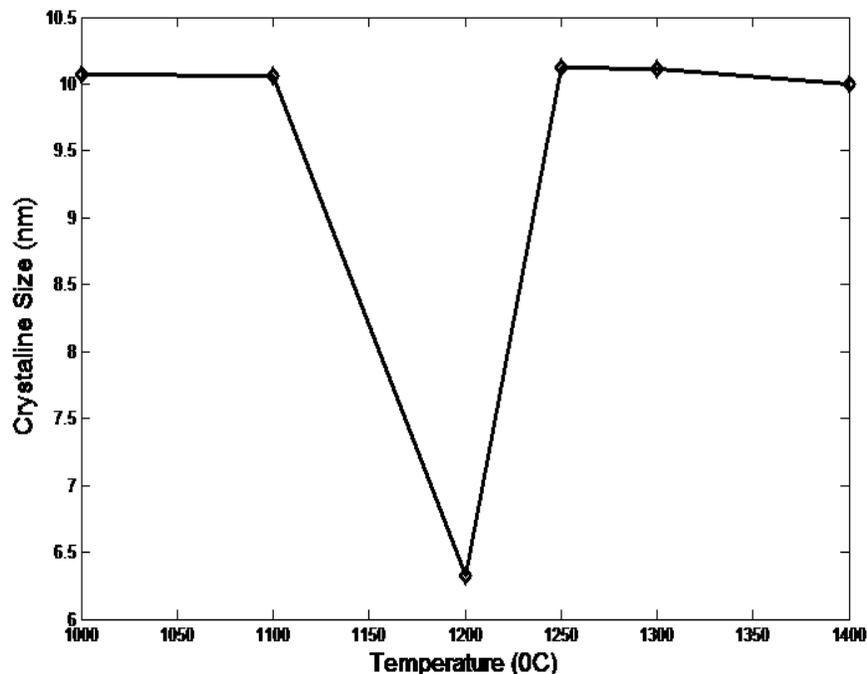
Fig2. Plot of Crystallite Size against Sintering Temperature
