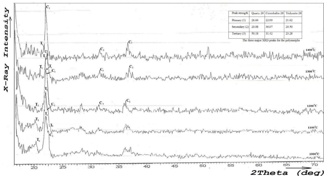
Fig. 1 X-ray Diffractograms for RHA Refractory in Temperature range 1000 °C to 1400 °C (The symbols C and T are peak positions for Cristobalite and Tridymite respectively)
