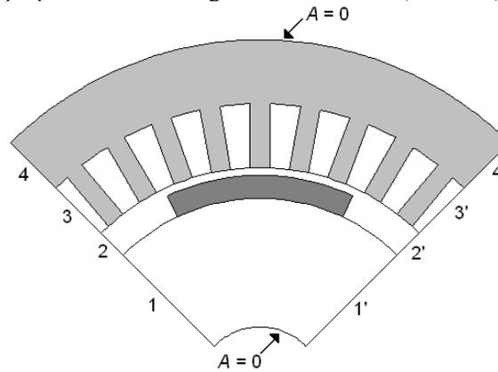
Figure 3. Boundary conditions for a four-pole dc motor.
