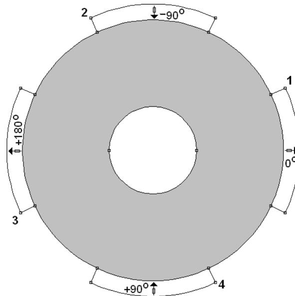
Figure 6. Permanent magnets 1, 2, 3 and 4 magnetized in a set direction.
