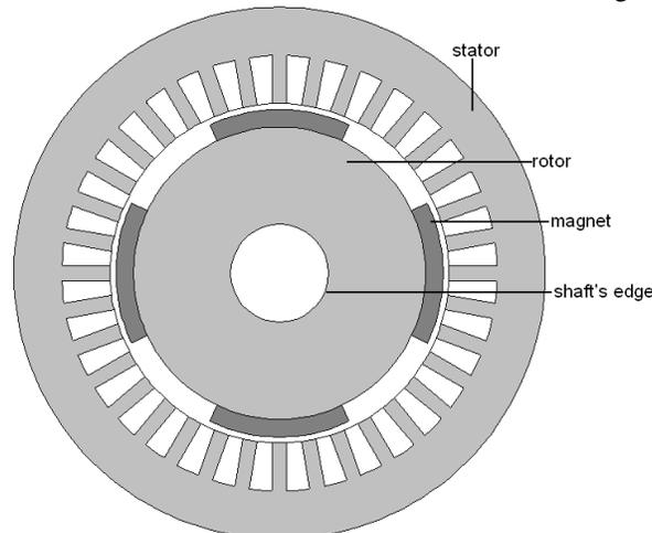
Figure 1. Cross-sectional view of a *dc* surface-mounted permanent-magnet motor.
