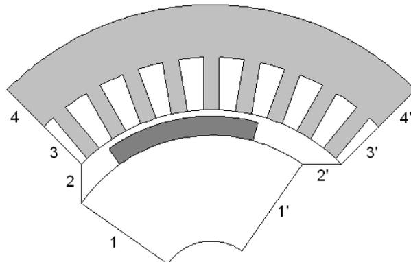
Figure 4. Field problem that represents a  $10^\circ$  rotation of the rotor in the counter-clockwise direction.
