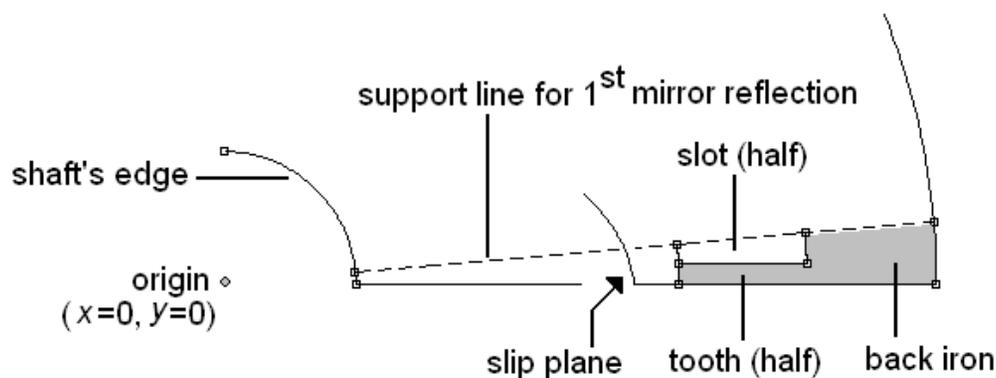
Figure 5. Elementary cell for the stator.
