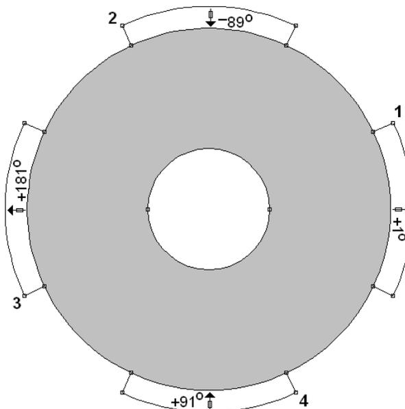
Figure 7. Redefinition of magnetization directions for magnets 1, 2, 3 and 4.
