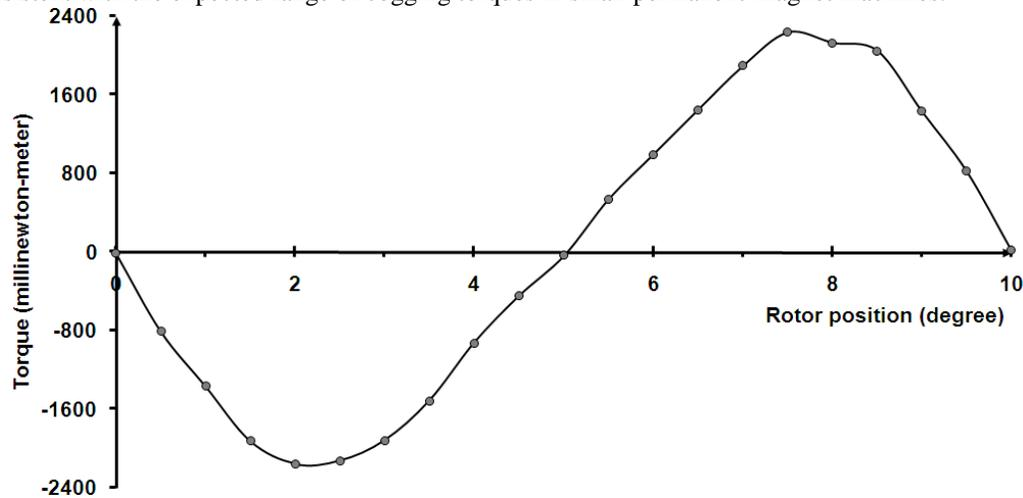
Figure 9. Cogging torque characteristic for the test motor.
