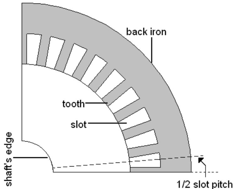
Figure 2. Regions for the construction of the model.
