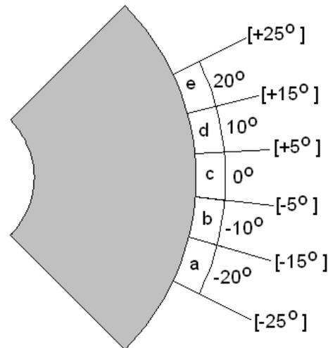
Figure 8. Magnetization directions for radially-oriented permanent magnets.
