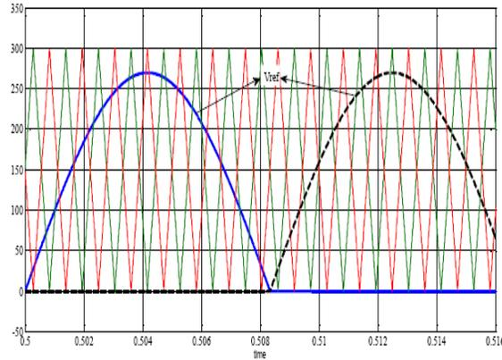
Fig.7: Sine triangle PWM for split natural balancing
