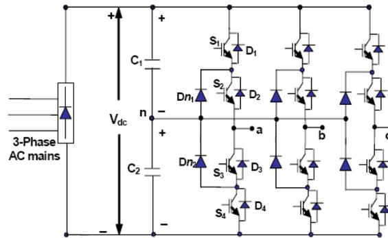
Fig.3: Three-level neutral-point clamped inverter topology
