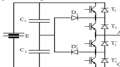
Fig.2: Three-level Capacitor-Clamped Multilevel inverter
