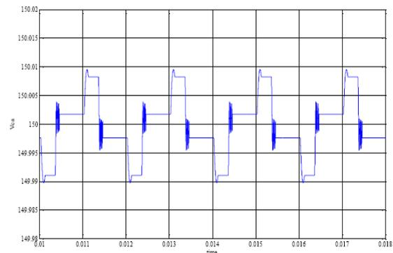
Fig8: Output waveform quality of the 3-level inverter (Capacitor voltage  $V_{ca}$  at PF=0.9)
