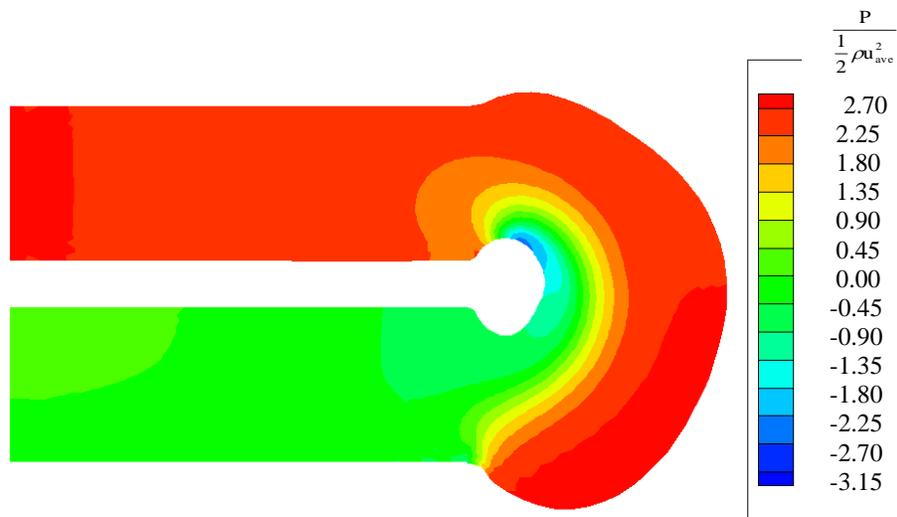
Figure 12 Pressure contours of the flow inside optimized shape of the channel
