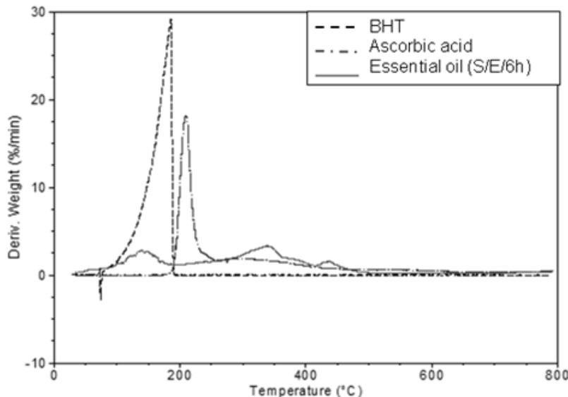
Figure 3. Derivative thermogravimetric curves of oregano essential oil obtained by Soxhlet with ethanol for 6 h, BHT and ascorbic acid.
