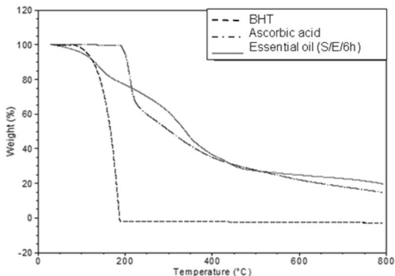
Figure 2. Thermogravimetric curves of oregano essential oil obtained by Soxhlet with ethanol for 6 h, BHT and ascorbic acid.
