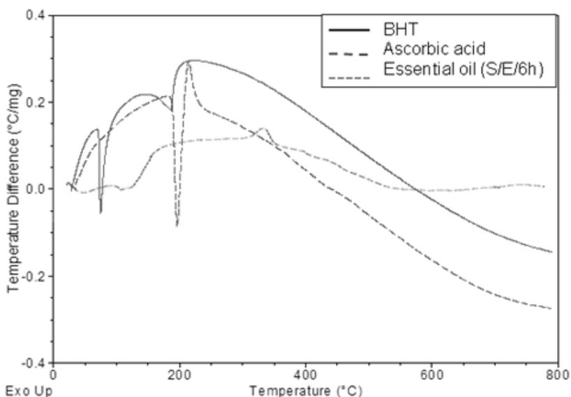
Figure 4. Differential thermal analysis curves of oregano essential oil obtained by Soxhlet with ethanol for 6 h, BHT and ascorbic acid.
