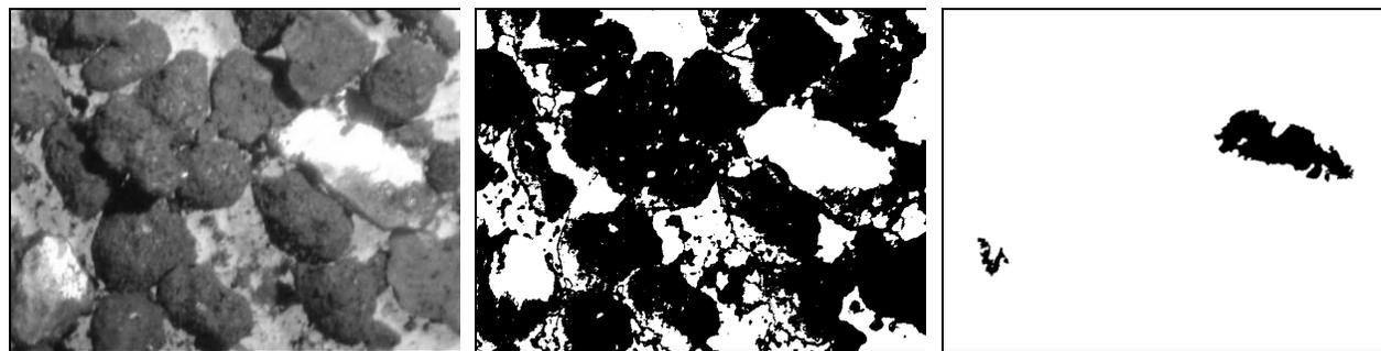
Figure 3. Digital image analysis results: (a) sample digital image to be analyzed, (b) results for minerals in Group A and (c) results for minerals in Group C.
