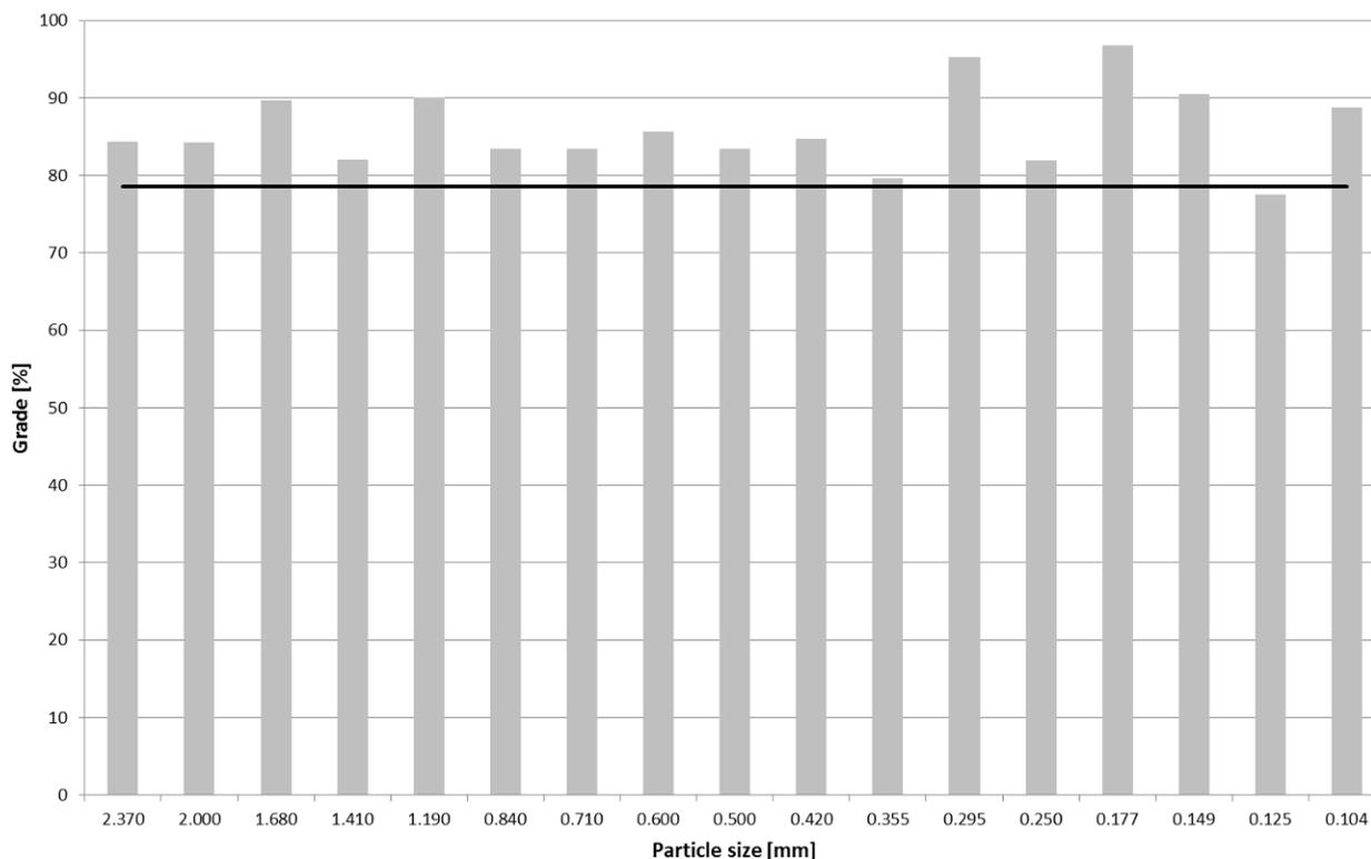
Figure 5. Estimated grade for each particle size (represented by gray bars) versus chemical grade (represented by a dark line).
