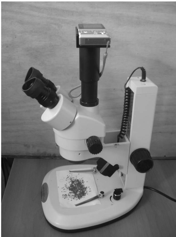
Figure 2. Assembly used to acquire the digital images: Sony DSC-S730 (7.2 MP) camera coupled into a Diagtech stereo microscope ZOOM 645.
