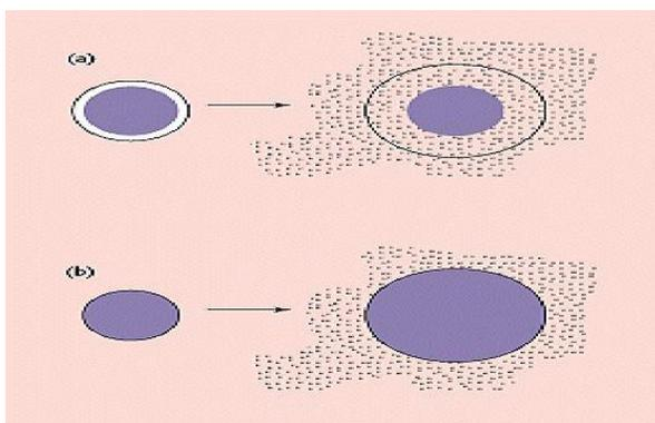
Figure 5 (a) shows reservoir diffusion swelling and (b) show matrix diffusion swelling [18].
