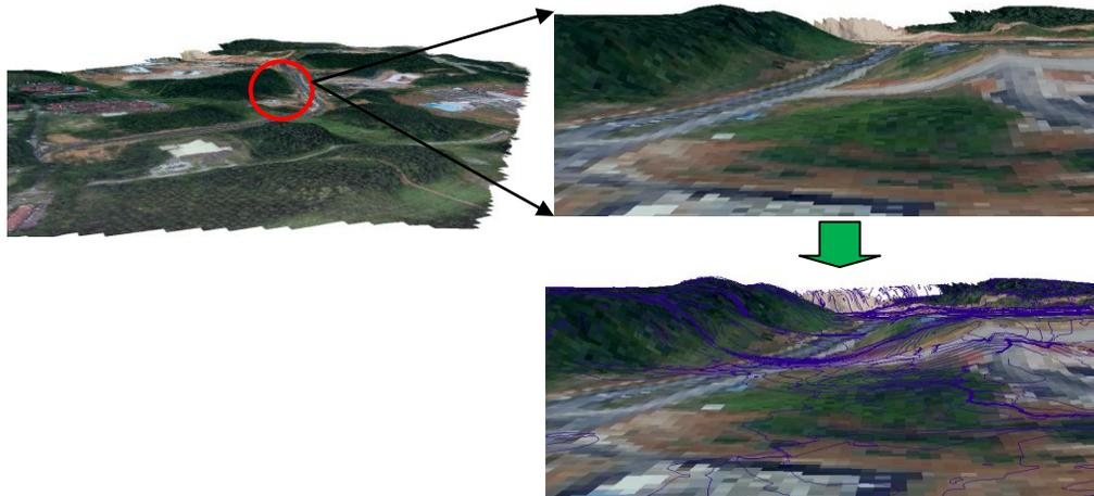
Figure 5. Superimposition of digital orthophoto, DEM and contour
