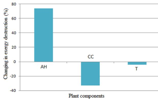
Figure 7. Change in exergy destruction in components due to 120% increase in the turbine inlet temperature
