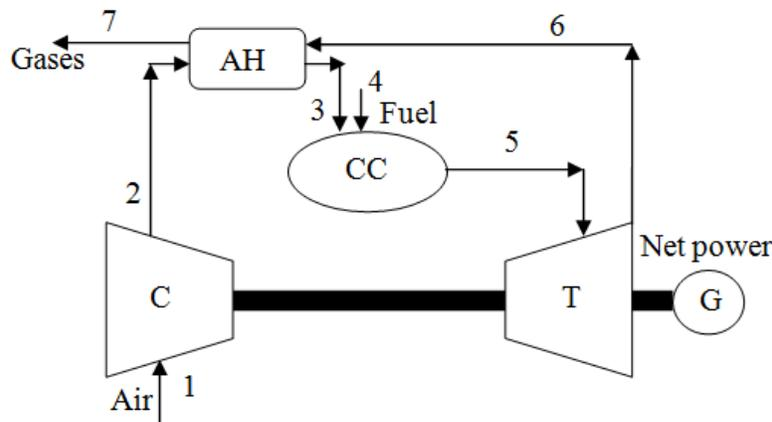
Figure 2. Air pre-heater gas turbine plant
