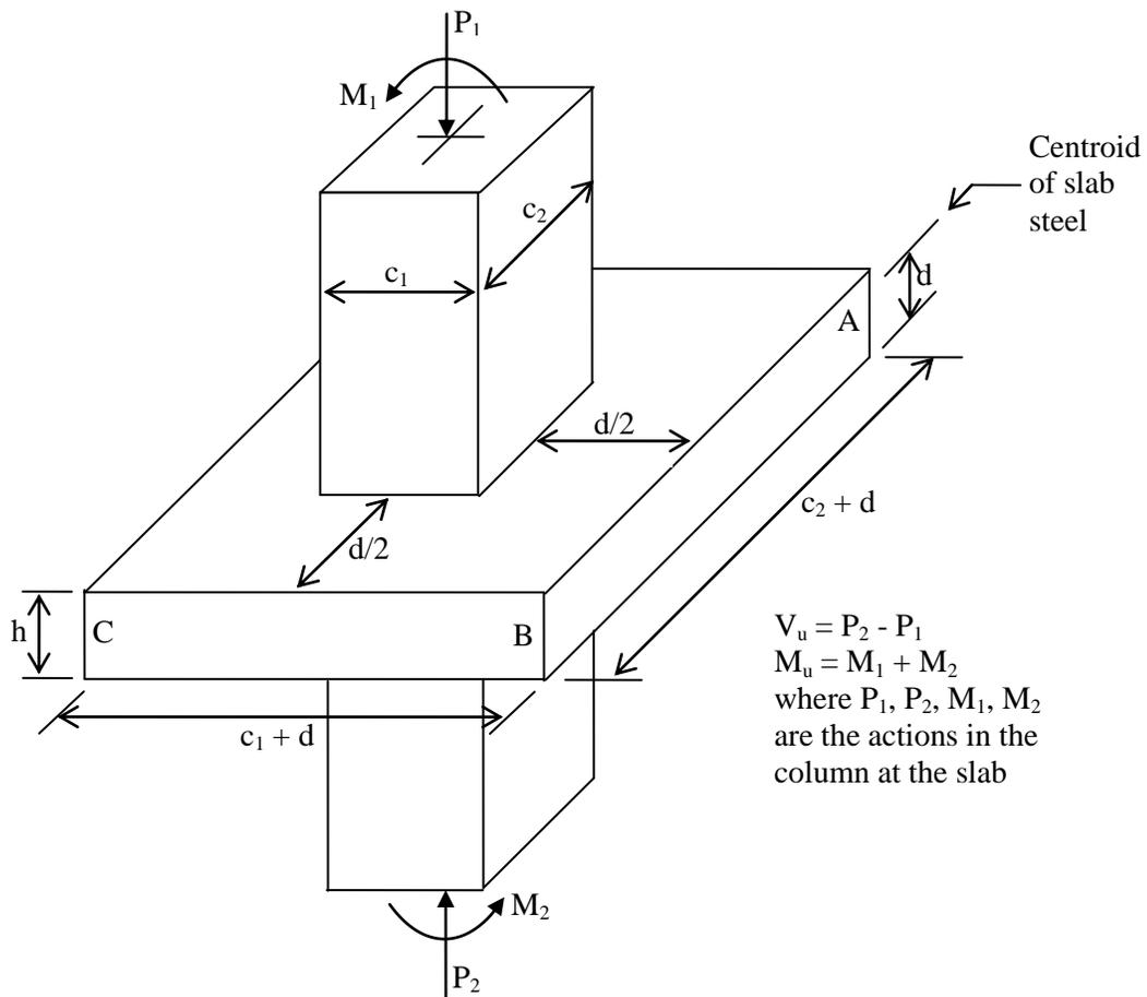
(a) External loads and the critical section at distance  $d/2$  from column face
