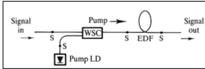
Figure 1: Forward pumped EDFA structure [3]
