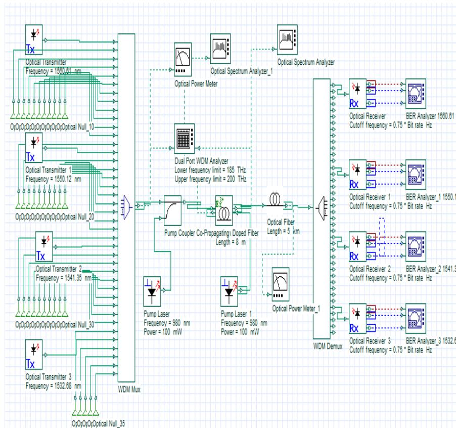
Figure 5: Basic simulation setup
