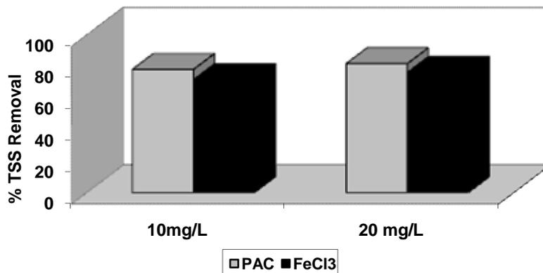
Figure 5: Removal of TSS by ferric chloride and PAC in different concentrations
