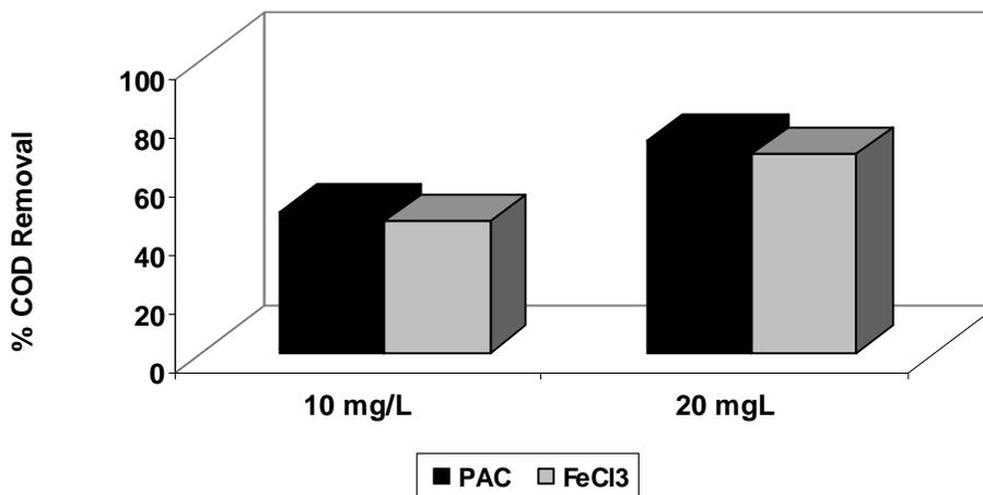
Figure 4: Removal of COD by ferric chloride and PAC in different concentrations
