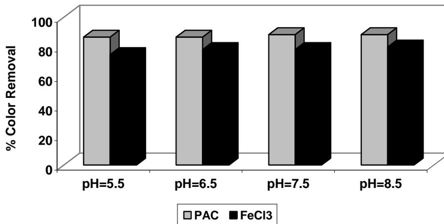
Figure 2. Effect of initial pH on color removal
