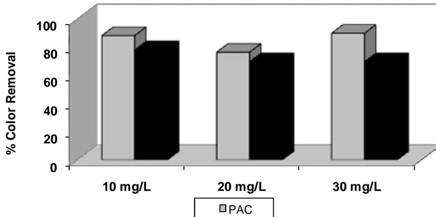
Figure 3. Effect of coagulant dose on color removal
