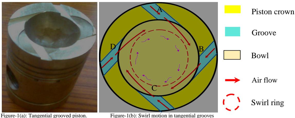
Figure-1(a): Tangential grooved piston.
