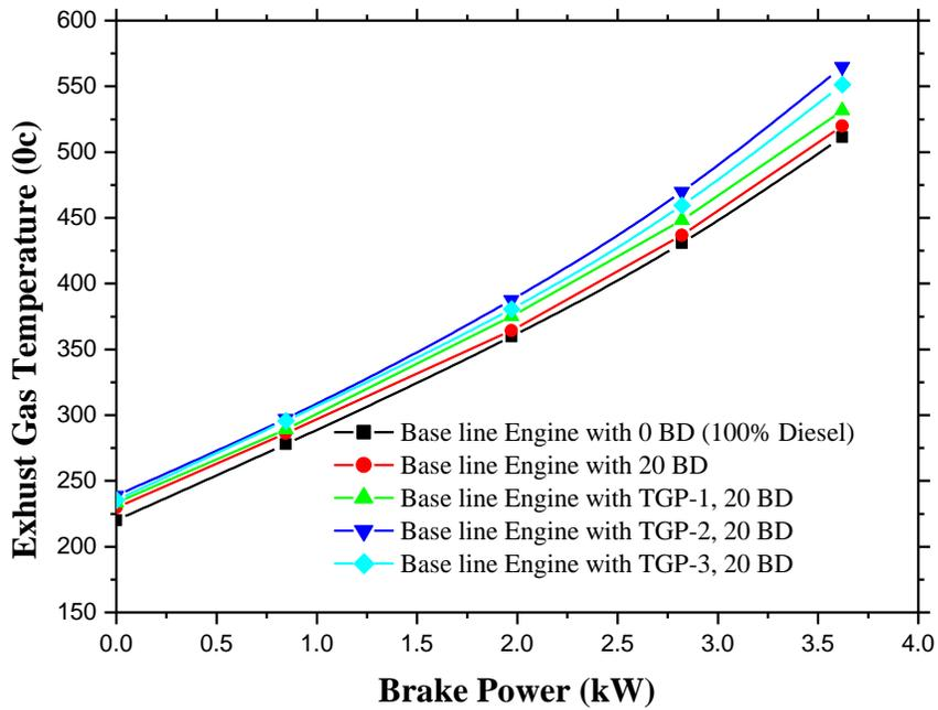
Figure-4: Brake Power vs EGT
