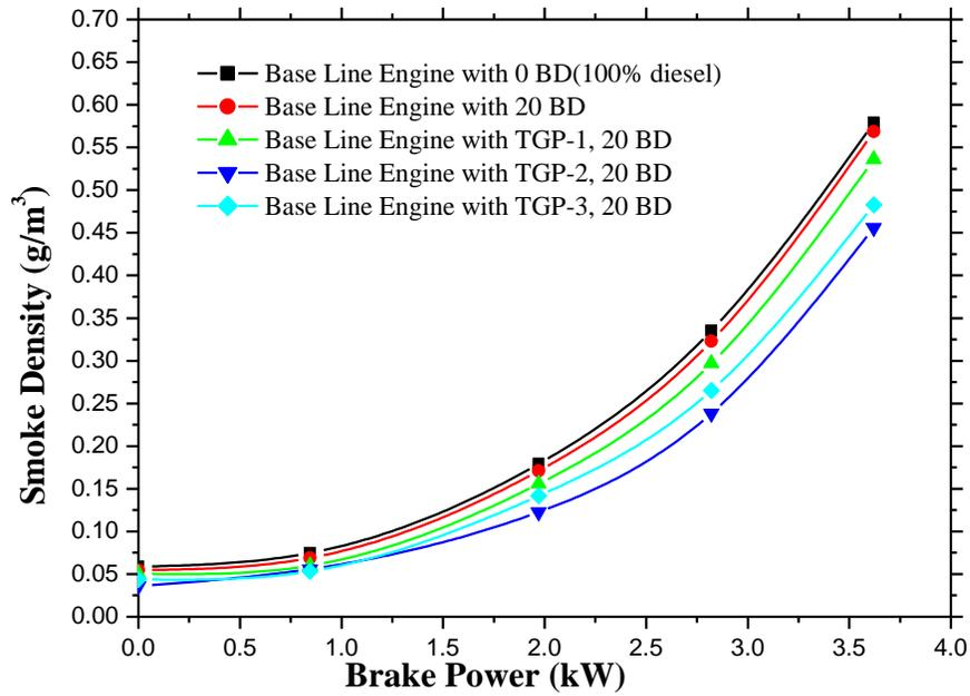
Figure-10: Brake Power vs Smoke Density
