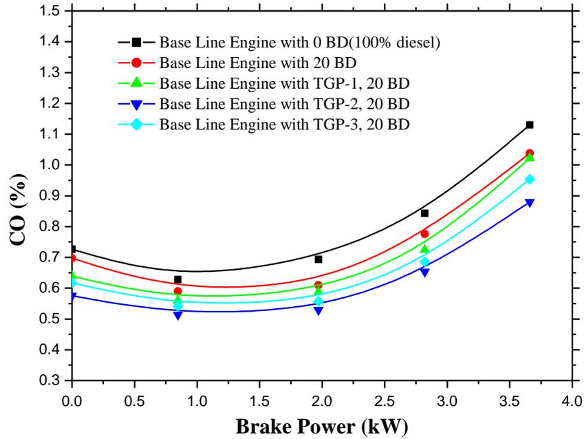
Figure-9: Brake Power vs Carbon monoxide
