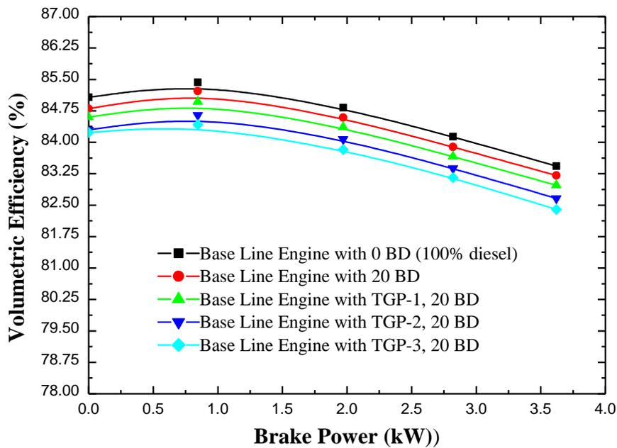
Figure-6: Brake Power vs Volumetric Efficiency
