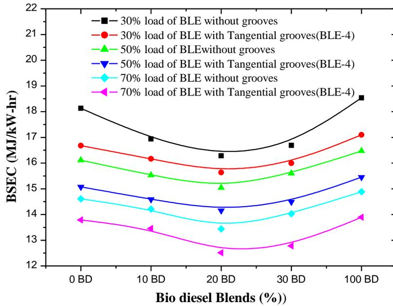
Figure-3: Bio Diesel Blends vs BSEC
