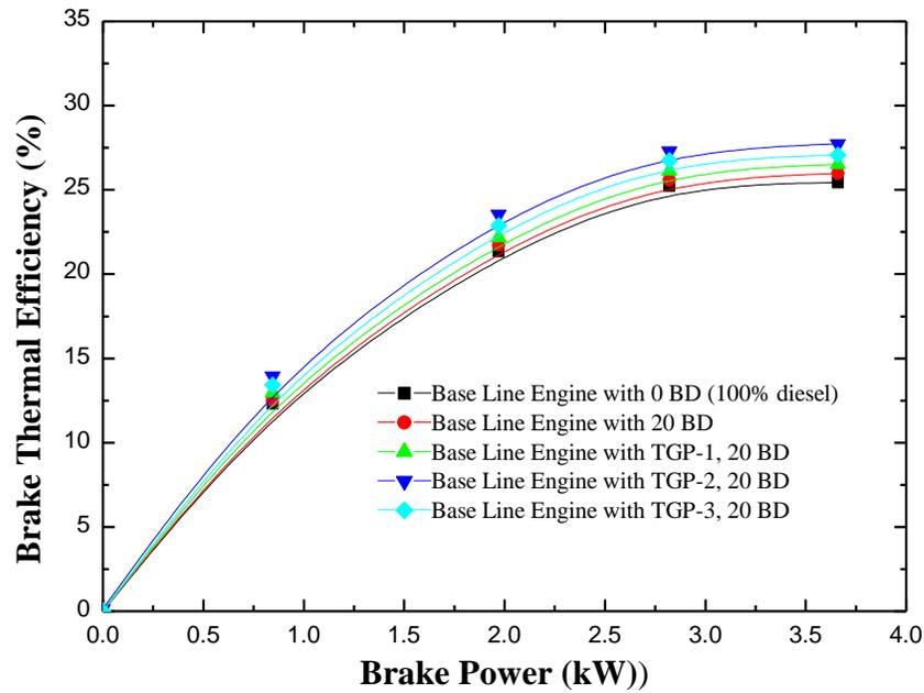
Figure-5: Brake Power vs Brake Thermal Efficiency
