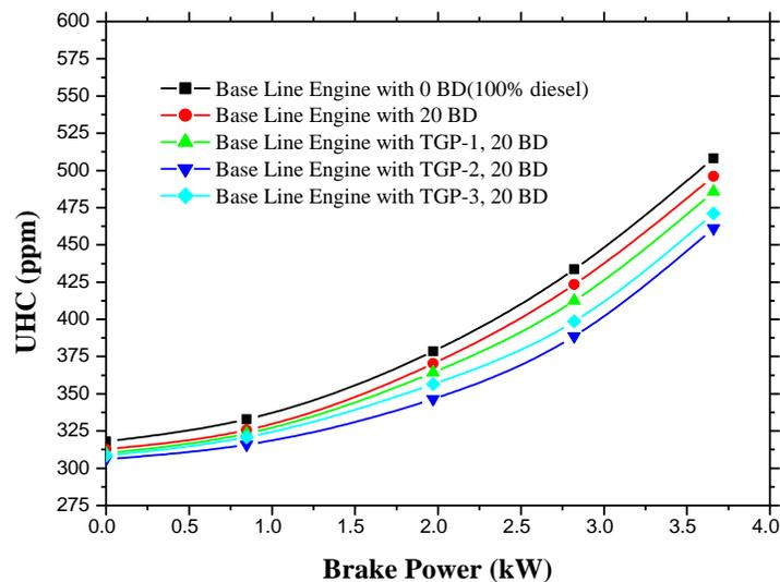
Figure-11: Brake Power vs Unburnt Hydrocarbons
