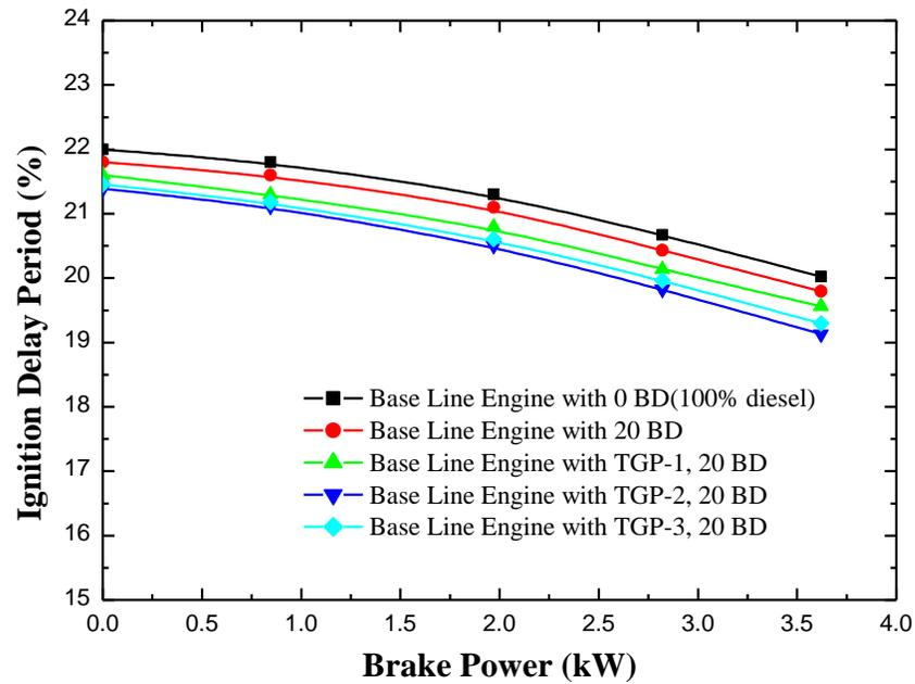
Figure-7: Brake Power vs Ignition Delay Period
