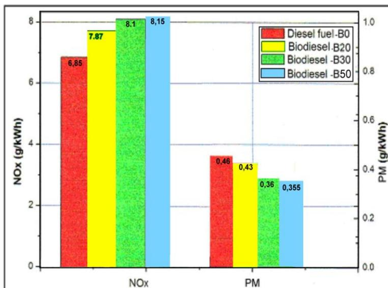
Figure 4. Specific PM and NO<sub>x</sub> emissions with four types of diesel fuels
