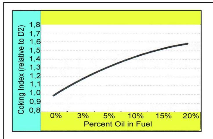
Figure 3. The tendency to form carbon deposits as function of percent vegetable oil into diesel fuel
