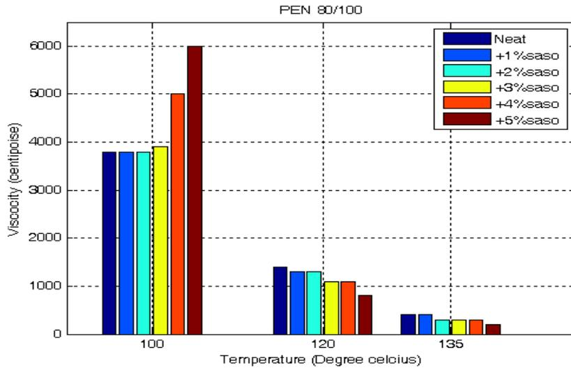
Figure 2: PEN 80/100 Viscosity measured at a shear rate of 6.8/s
