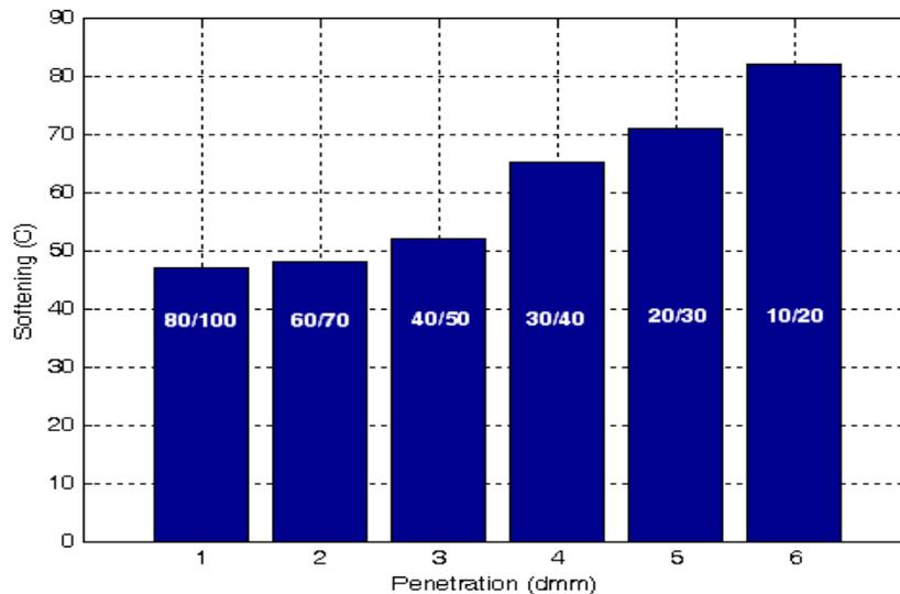
Figure 3 ; The softening point and penetration of bitumen with various additive content
