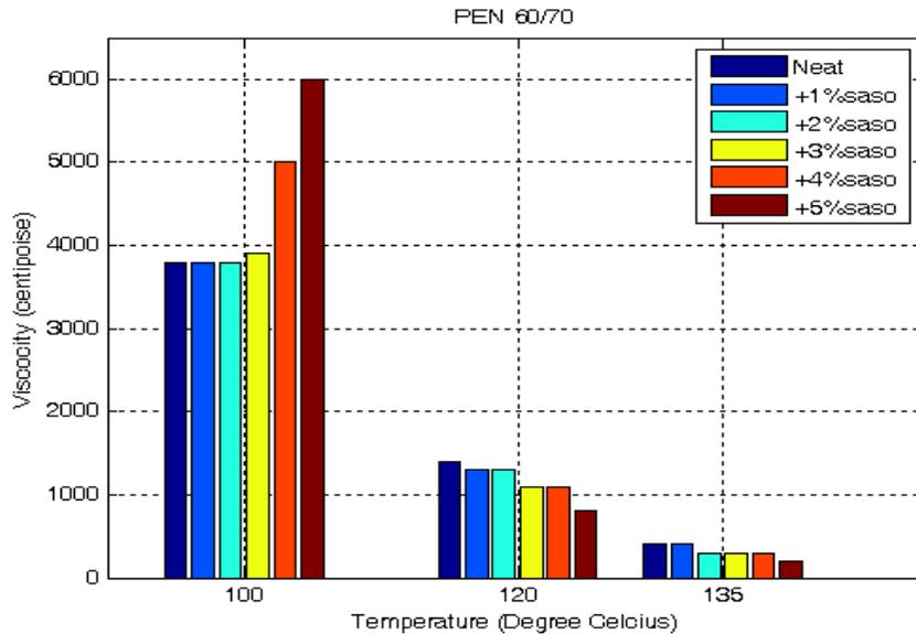
Figure 1: PEN 60/70 Viscosity measured at a shear rate of 6.8/s
