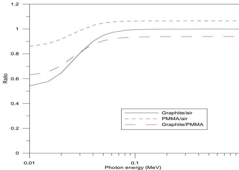
Fig. 5: Variation of relative attenuation coefficient with X-ray energy.
