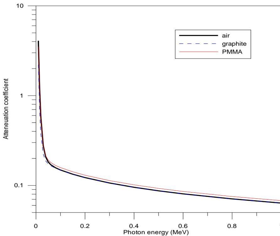
Fig. 4: Attenuation coefficient of graphite, PMMA and air versus X-ray energy.
