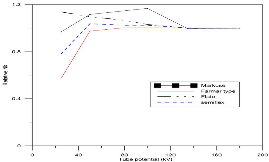
Fig. 3 Relative  $N_K$  of ion chambers used as a function of X-ray  $K_p$ .
