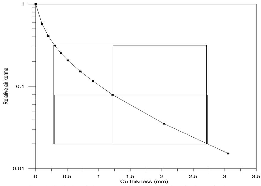
Fig. 1: Relative air kerma as a function of filter thickness in Cu.
