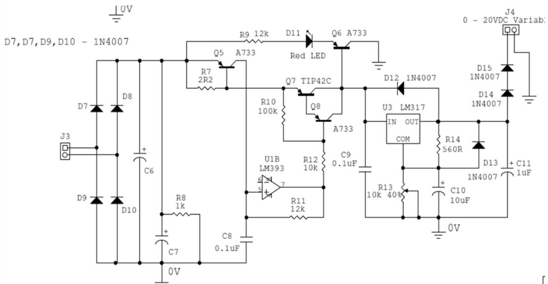
Figure 4: Circuit Diagram for Variable DC Circuit
