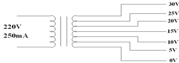
Figure 2: Circuit Diagram for AC Regulated Output
