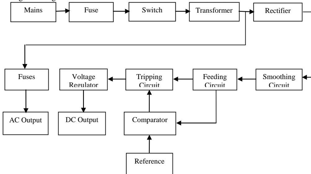
Figure 1: Block diagram of a multi-output power supply
