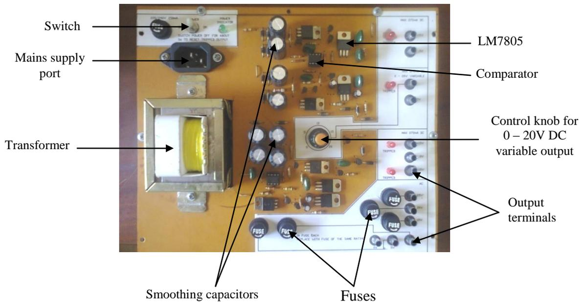
Figure 6: Final construction of the power supply unit
