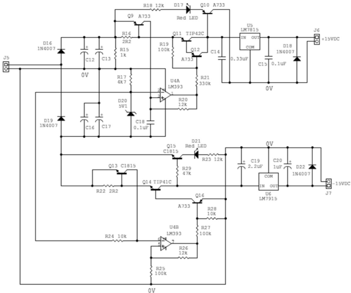
Figure 5: Circuit Diagram for Regulated DC Dual Rectified Circuit
