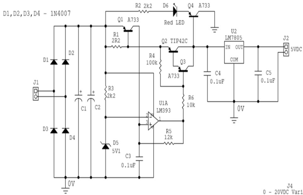
Figure 3: Circuit Diagram for Regulated DC Circuit
