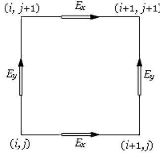
Figure 1: Lee discretization. Here  $H_x = (\nabla \times \bar{A})_x$ ,  $E_x = -(\partial(1+T\nabla \times) \bar{A} / \partial t)_x$  and with  $\bar{J} = 0$  (See [10-12, 17]).
