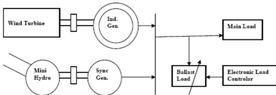
Figure 1. System configuration of the embedded generation
