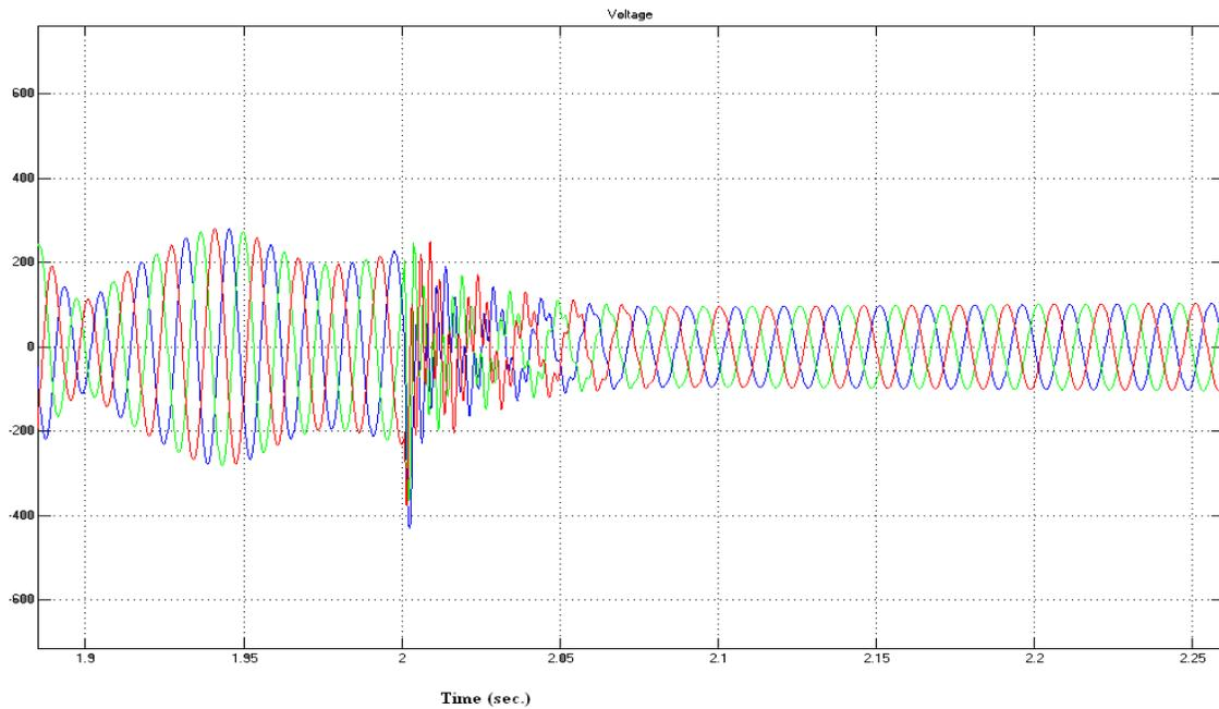
Figure 9. Voltage dip at the connection and disconnection of wind energy system
