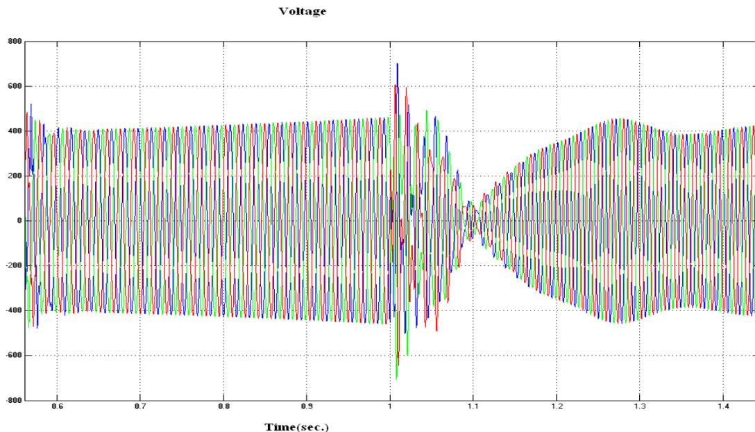
Figure 6. Voltage dips at the connection and disconnection of wind energy system
