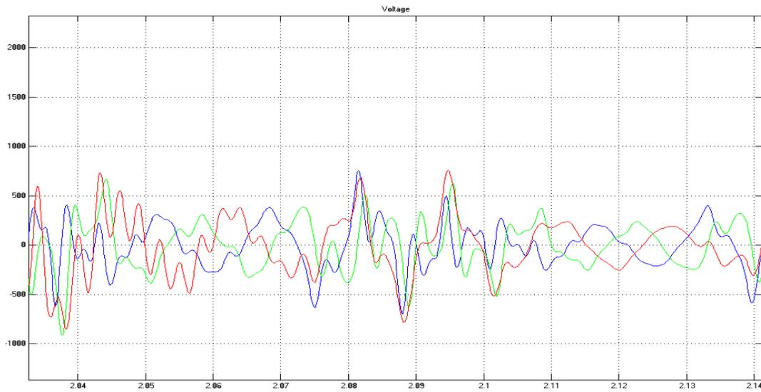
Figure 11. Voltage unbalancing due to unbalanced supply
