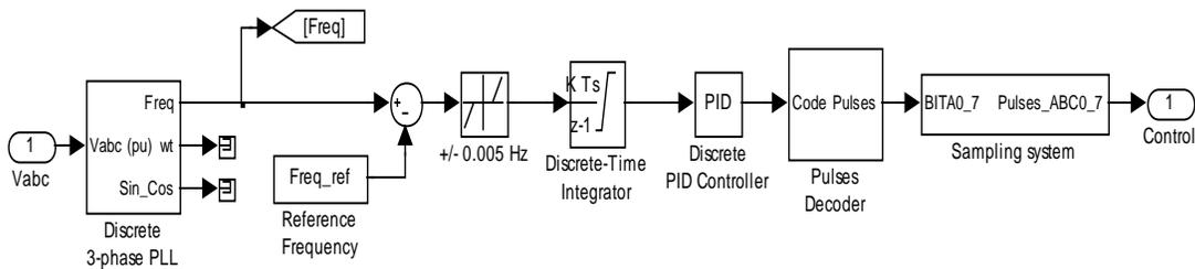
Figure 5. Discrete frequency regulator
