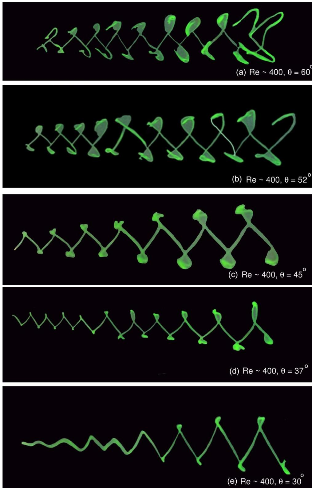
**Fig. 3** Top view. Variation in the shape of the vortices as a function of angle of attack. These vortices were generated using the long, stainless steel needle (Table 1) and look more stable and robust at  $\alpha = 45^\circ$  observed. Detailed studies by means of flow visualization showed that the resulting flow was three-dimensional and providing stable vortex shedding below  $Re = 700$ .
