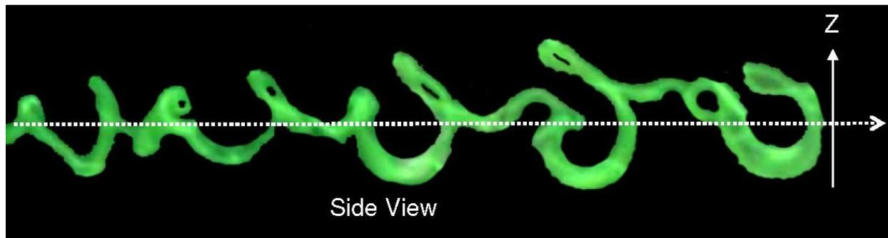
**Fig. 5** Side view of the K-type vortices using the big plastic needle (Table 1). In this experiment,  $Re$  was set at 700 and the angle of attack was  $45^\circ$ .
