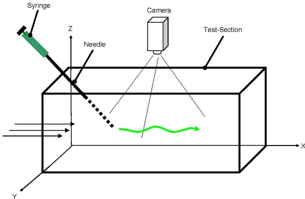
**Fig. 2** Schematic view of the experimental recirculating water-tank facility used in this study. Note that the diagram is not to scale.
