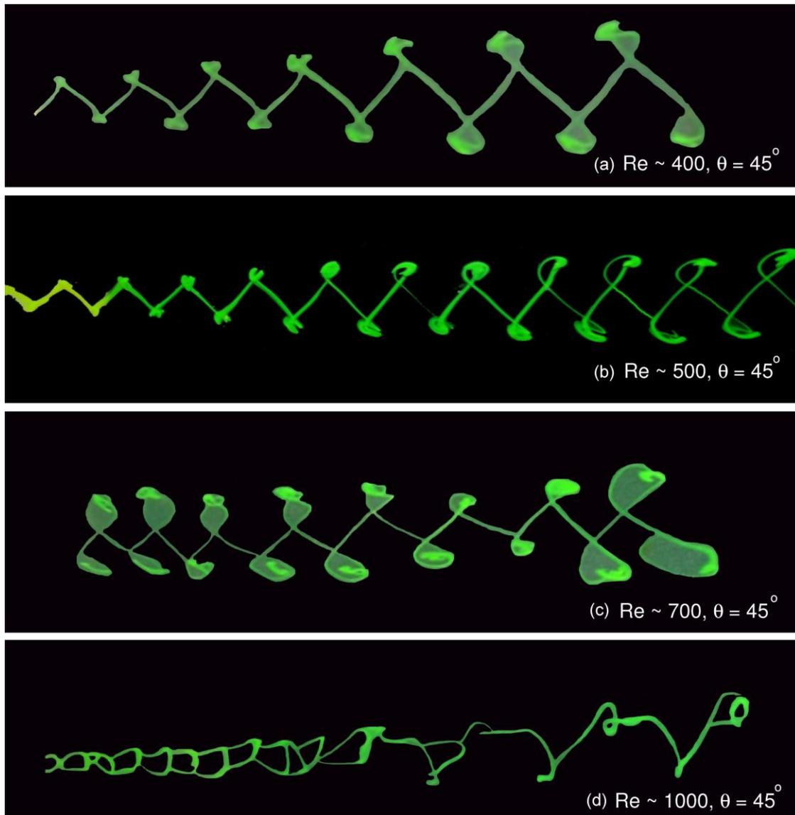
**Fig. 4** Top view. Alteration in the shape of vortices as a function of  $Re$  and fixed angle of attack. Three different states could be distinguished: the development of non-axisymmetric periodic vortex shedding ( $Re < 700$ ), transition from periodic vortex shedding to chaotic motion which comprises distorted vortices ( $700 > Re > 1000$ ), and a state in which the vortices disappear because of  $Re$  ( $Re > 1000$ ).
