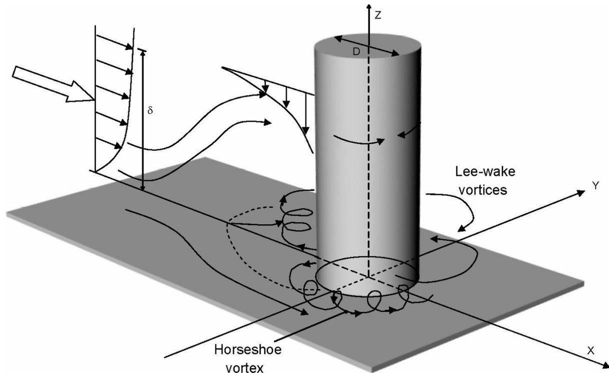
**Fig. 1** Definition sketch for flow past vertical cylinder.
