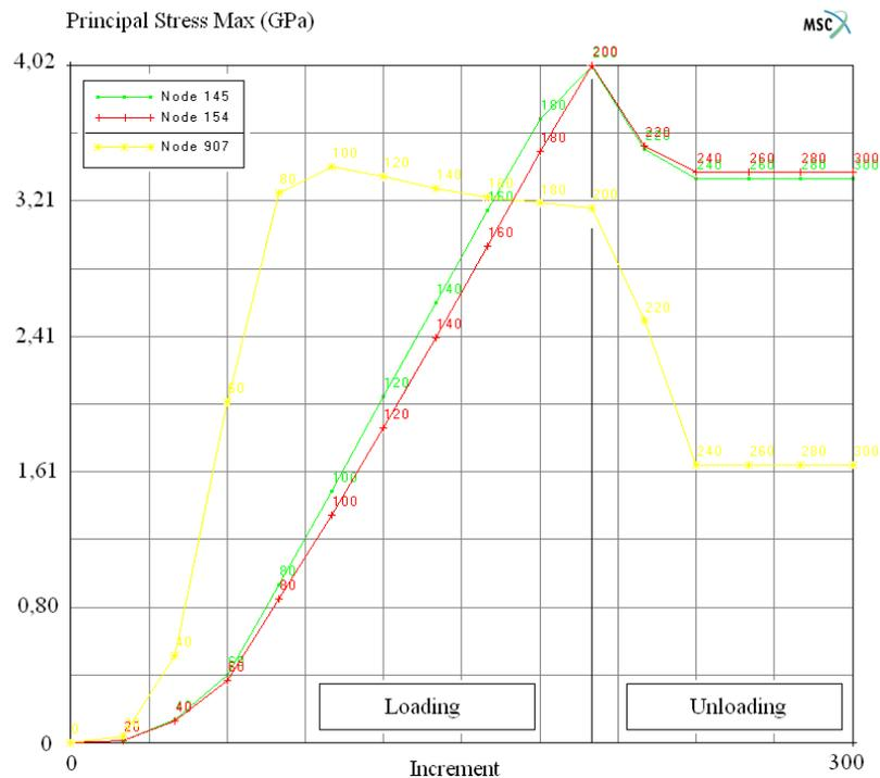
Figure 7. Numerical evolution of highest principal stress during indentation testing in CrN with fifteen micrometres thickness deposited in soft substrate.
