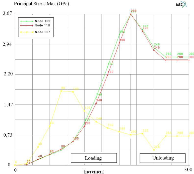
Figure 6. Numerical evolution of highest principal stress during indentation in CrN with fifteen micrometres thickness deposited in hard substrate.
