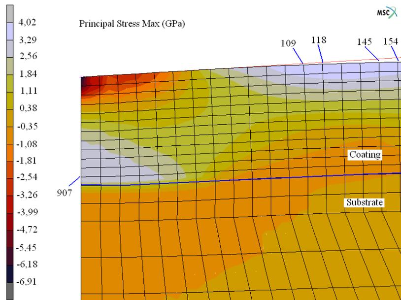
Figure 5. The Maximum Principal Stress distributions in the contact area of the indenter.
