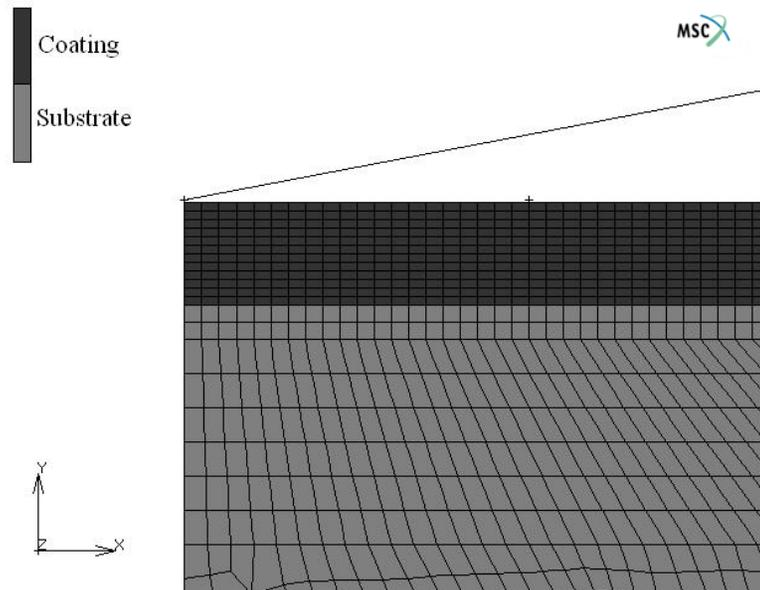
Figure 1. Detail of the numerical model mesh close to the indentation area.
