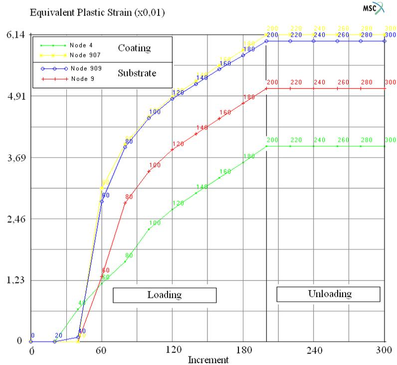
Figure 2. Numerical evaluation of plastic strain during indentation cycle for the CrN film with 15 μm thickness.
