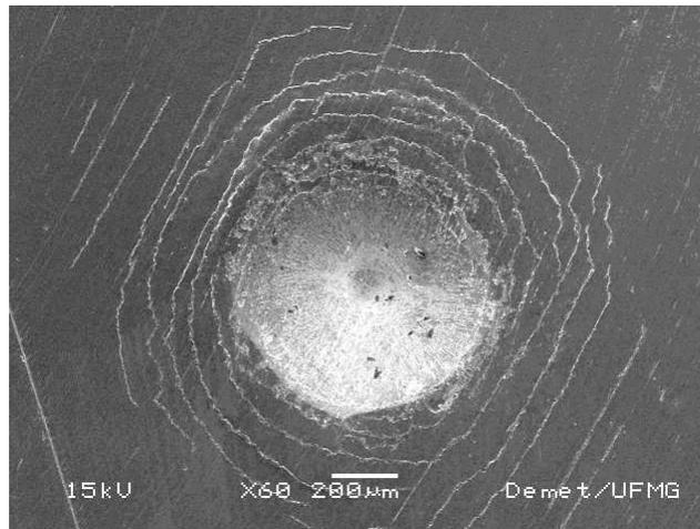
Figure 4. Circular and radial cracks around impression of spherical indenter [15].
