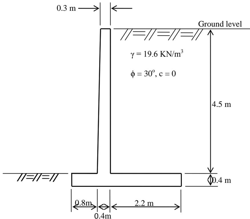
Figure 1. Schematic of reinforced concrete cantilever retaining wall
