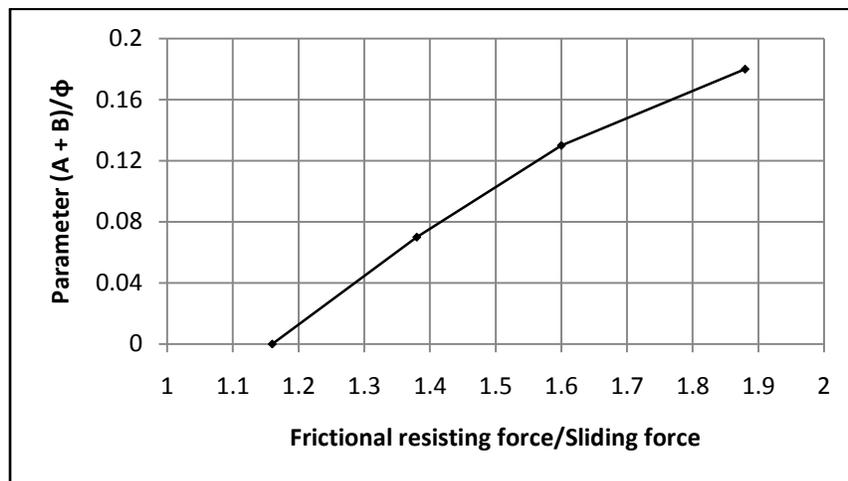
Figure 2. Relationship between design parameters (A, B, and  $\phi$ ) and factor of safety against sliding
