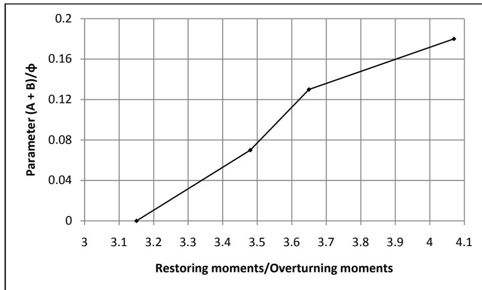
Figure 3. Relationship between design parameters (A, B, and  $\phi$ ) and factor of safety against overturning
