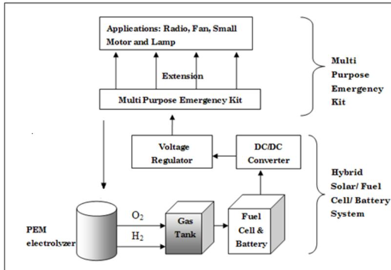
Figure 2 Schematic diagram of the HPSMEK device system
