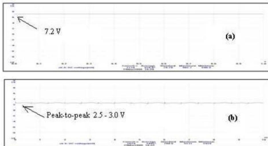
Figure 8. Pico-oscilloscope screen output showing performance characteristic of (a) Hybrid PEM fuel cell - lead acid battery without load (b) Hybrid PEM fuel cell- lead acid battery with load.
