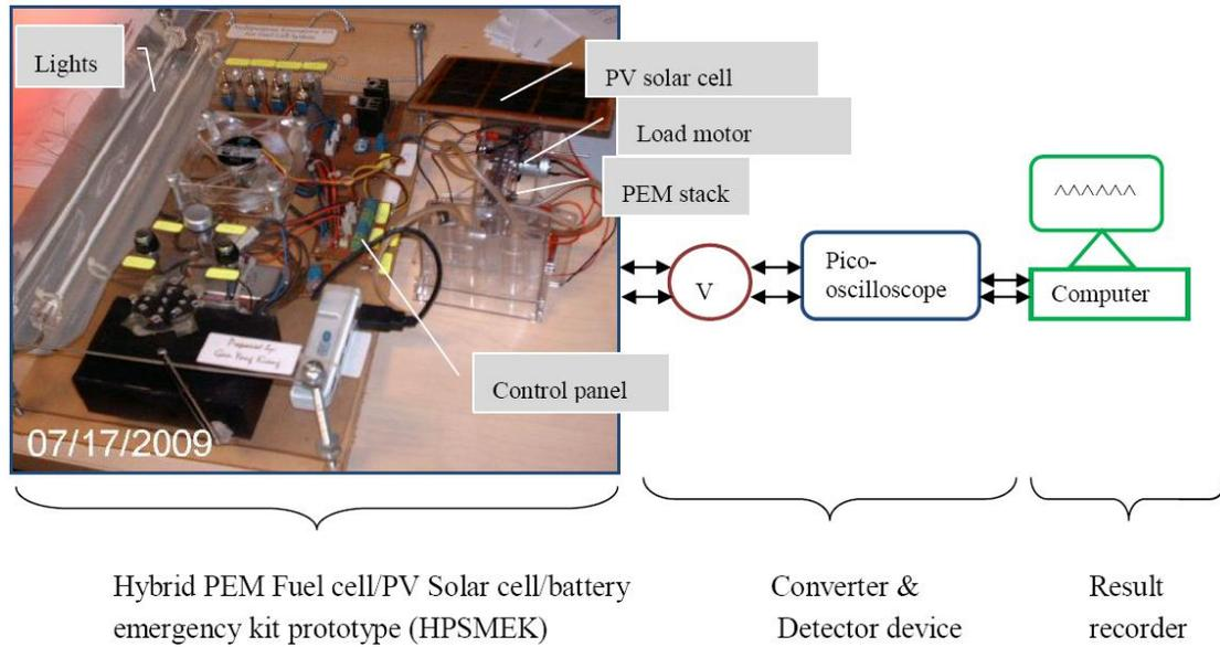
Figure 1 The prototype and the schematic of the associated experimental setup. The experimental rig essentially consists of three sections i.e. the prototype, converter & detector device and the computer result recorder.
