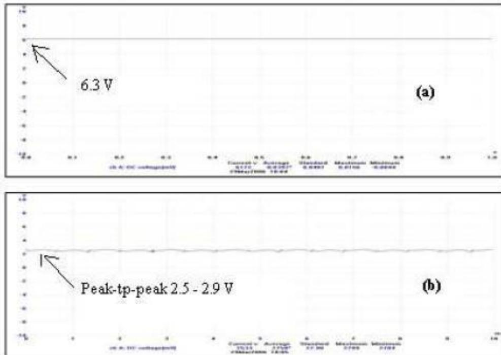
Figure 9. Pico-oscilloscope screen output showing performance characteristic of (a) Hybrid three power sources without load (b) Hybrid three power sources with load
