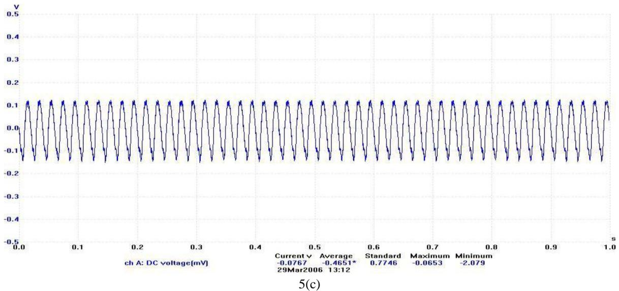
Figure 5. Pico-oscilloscope output showing the performance characteristic of (a) lead acid battery (b) PEM fuel cell; and (c) PV Solar cell, with load motor.
