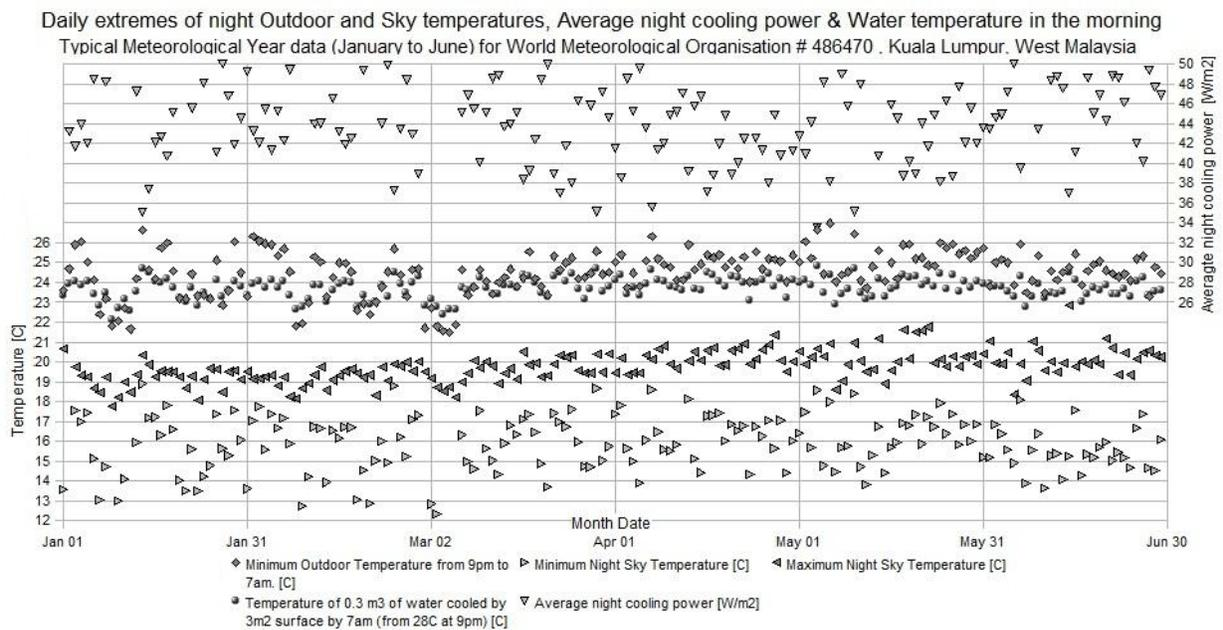
Figure 6. Night Outdoor and Sky Temperatures, Av. Cooling Power & Water Temperature in the morning, Jan to June.
