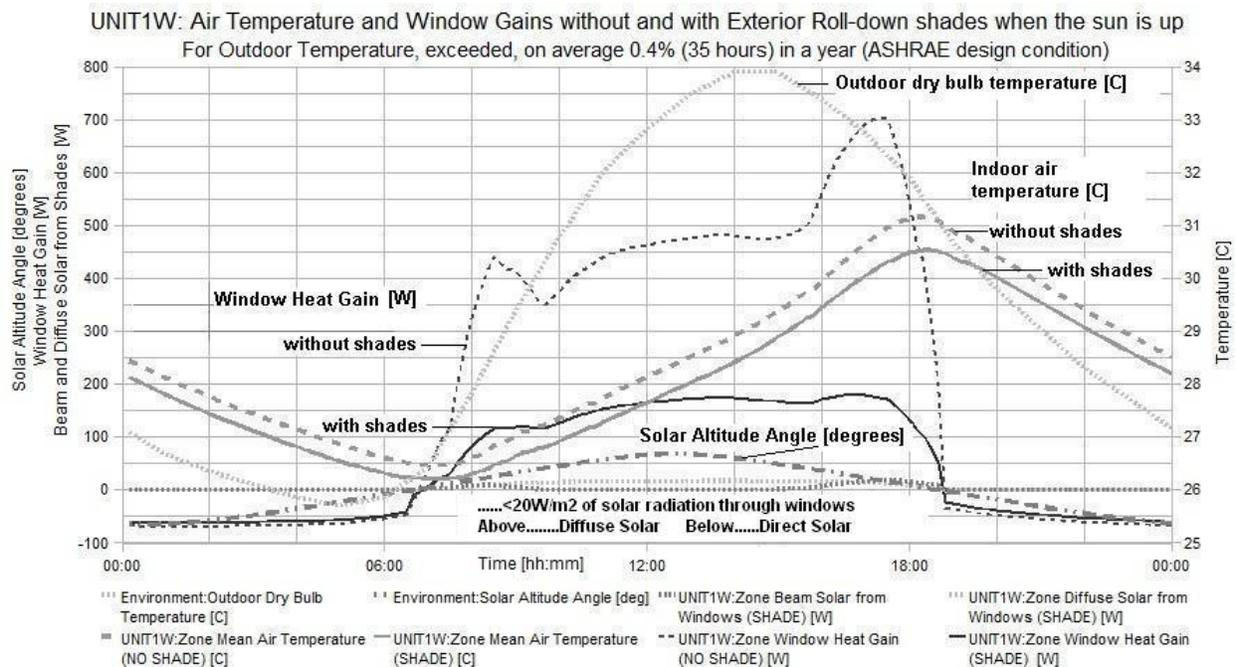
Figure 4. External Shades reduce the maximum indoor air temperature at 6pm from  $31.16$  to  $30.52^\circ\text{C}$ .
