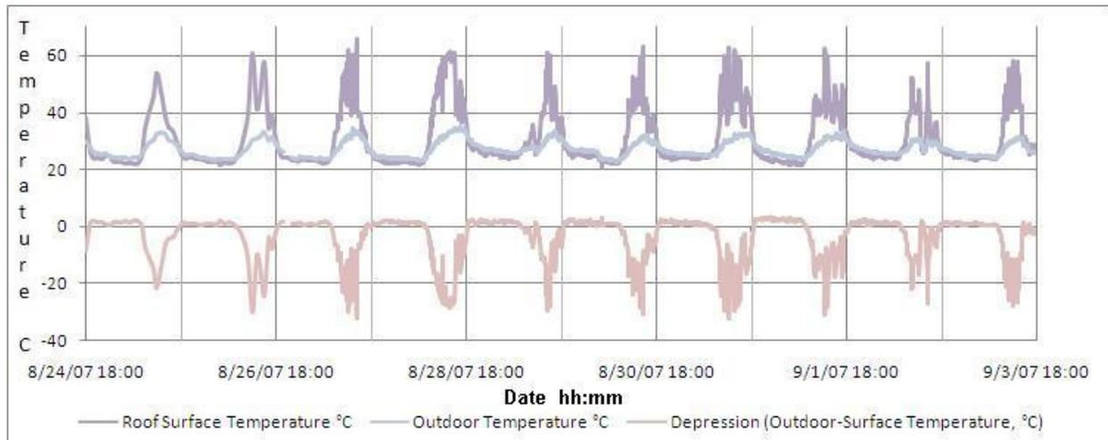
Figure 5. Measured Roof Surface and Outdoor Temperatures, Aug 2007.
