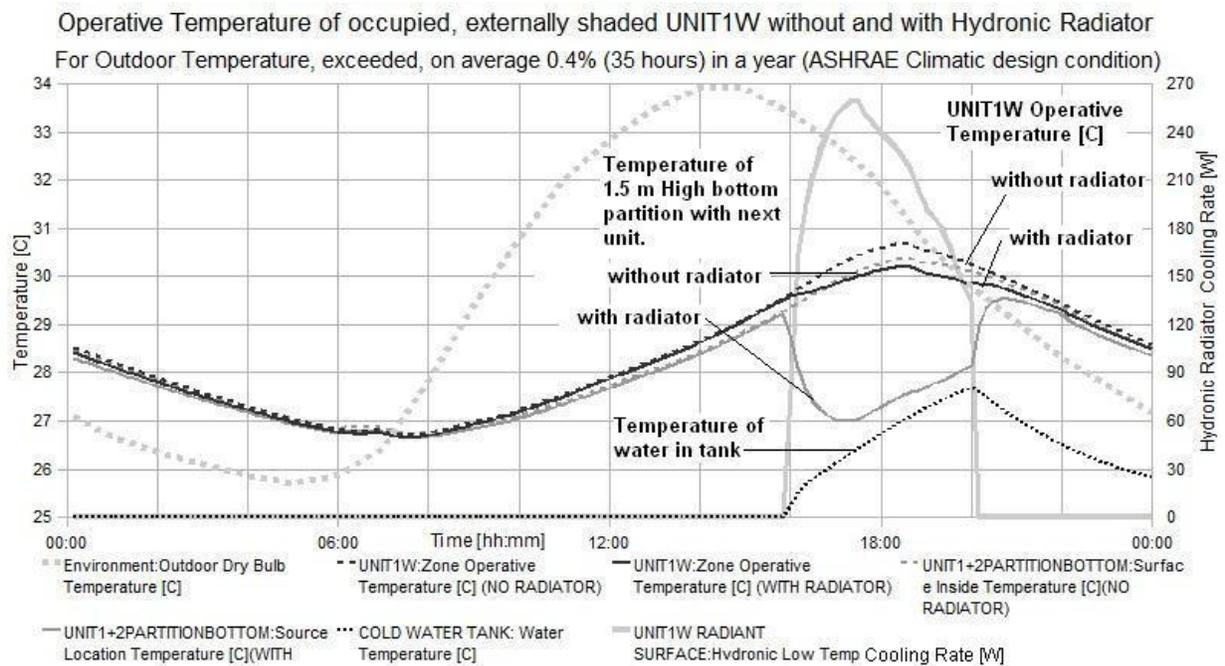
Figure 9. Effect of radiator on the operative temperature of an occupied externally-shaded low cost corener unit.
