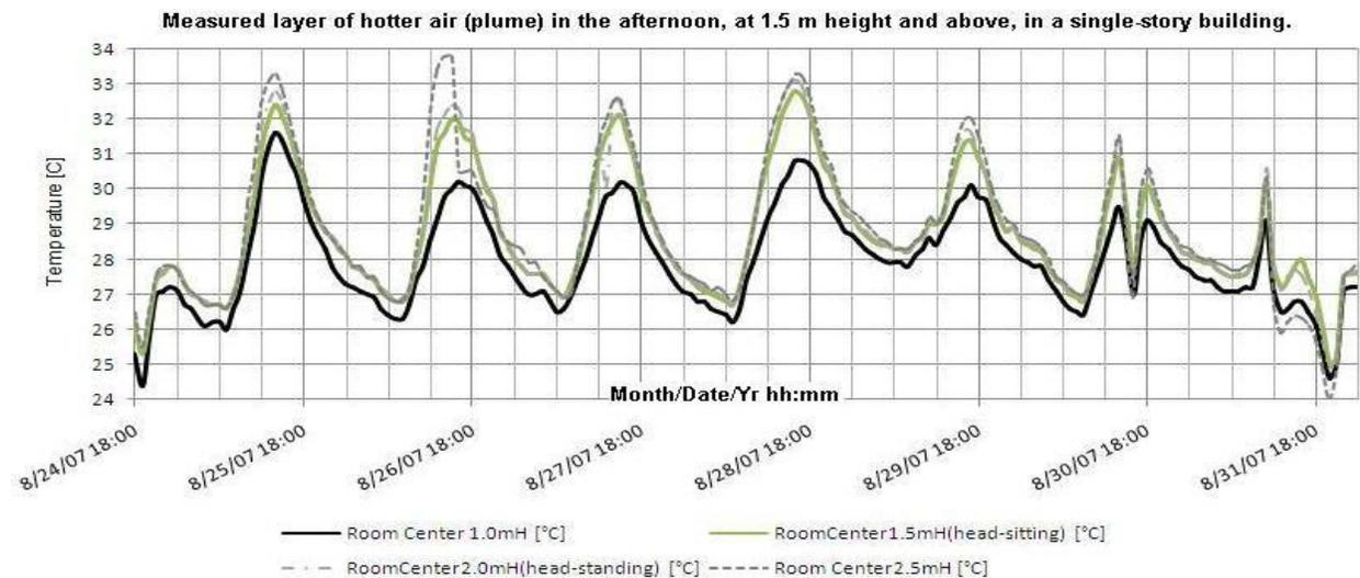
Figure 10. Measured indoor air temperatures at various heights in the center of a single story building, Aug 2007.
