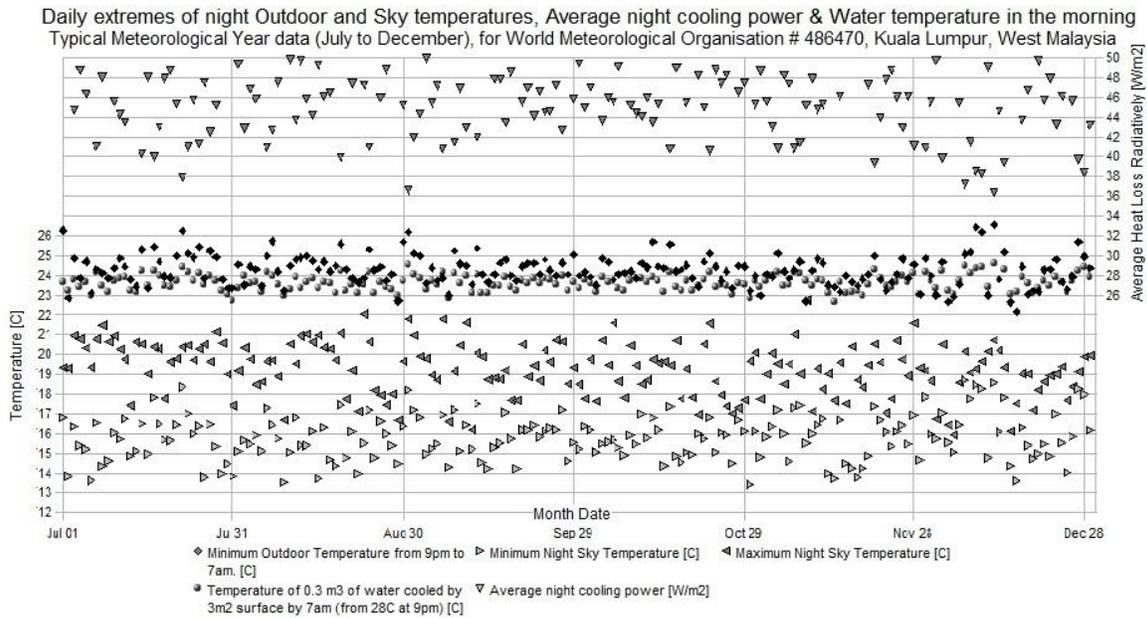
Figure 7. Night Outdoor and Sky Temperatures, Av. Cooling Power & Water Temperature in the morning, July to Dec.
