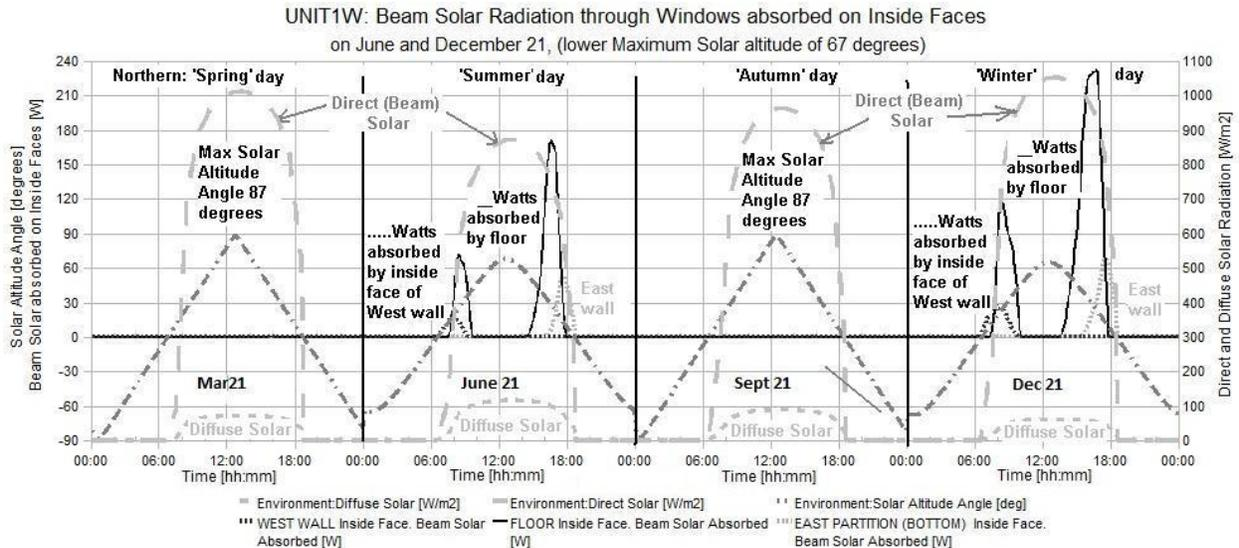
Figure 3. Radiation on floor, inside face of east and west walls from beam solar through windows on June & Dec 21.
